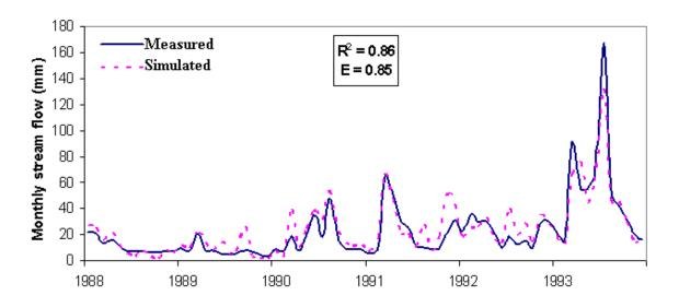
Figure 4. Monthly time series of predicted and measured streamflow at USGS gauge 05418500 (watershed outlet) for the 1988-93 calibration period
