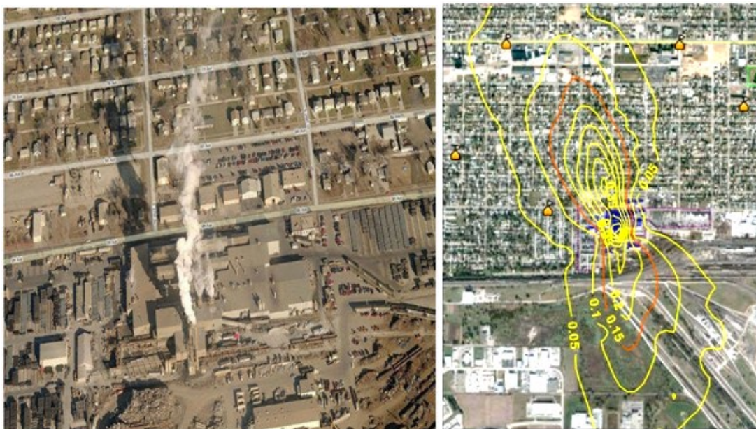
Local Air Pollutant Example. Industrial lead emissions (left) and modeled hotspot (right). Note that the image and the modeling results are no longer current. The area inside the orange contour was predicted to violate the NAAQS.
