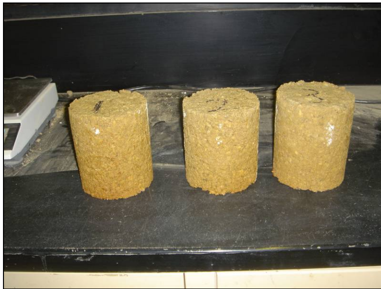
Figure 193. Soapstock-stabilized samples after vacuum saturation test
