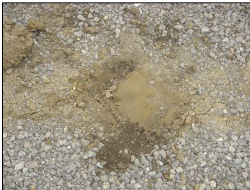
(a) Clay paleosol layer underlying granular layer
