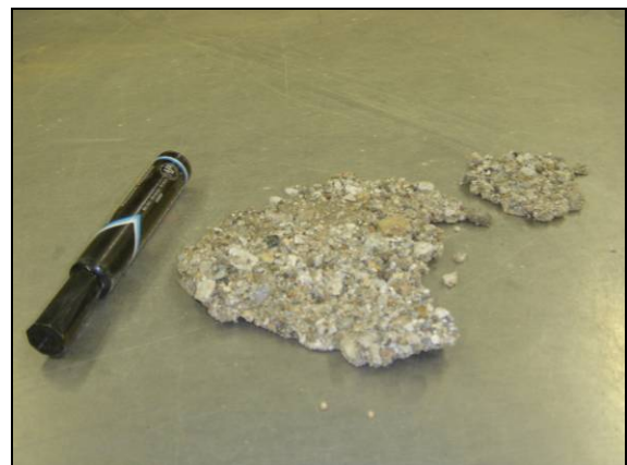
(b) Thin granular film forming on top of granular material
