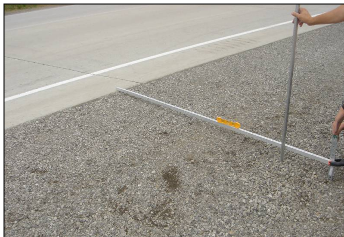
Figure 136. Determining shoulder elevations relative to the pavement, September 22, 2005
