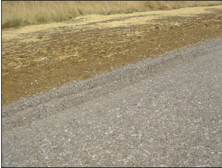
Figure 164. About 3 in. of rut developed after six passes
