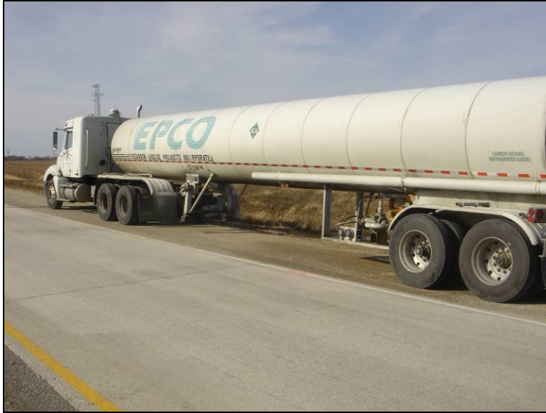
Figure 160. Stabilized shoulder along the exit ramp showing no rut under heavy traffic load, June 8, 2006
