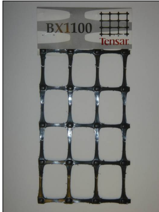
Figure 4. Tensar BX1100 geogrid (image scale 1:2.5)
