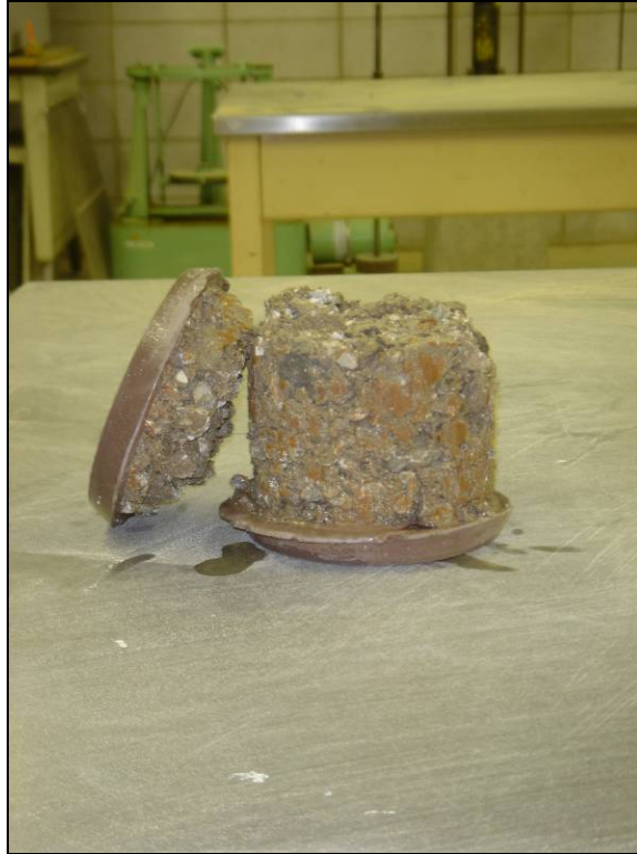
Figure 94. Disintegrated specimen after soaking for four hours
