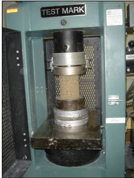
(a) Soiltac-stabilized sample
