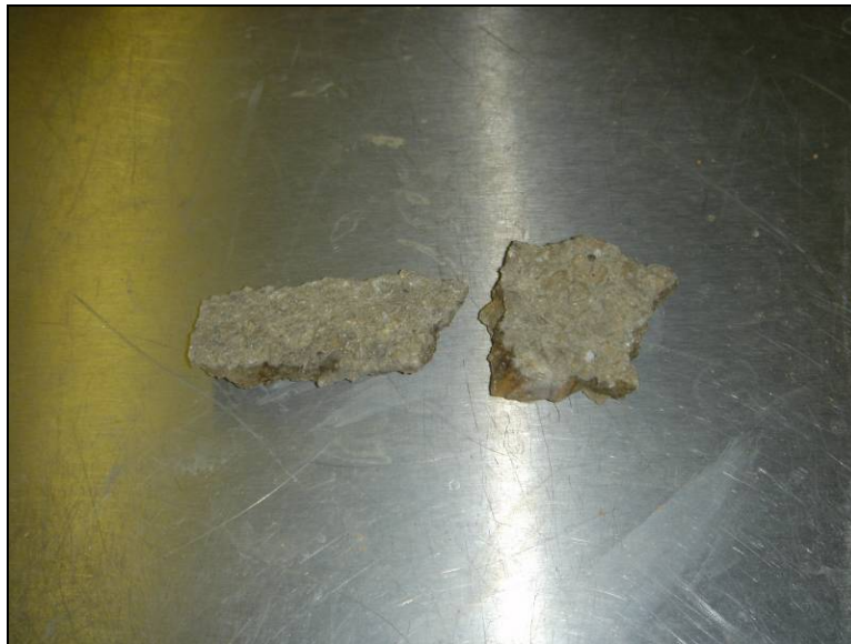
Figure 27. Crushed limestone samples stabilized with soybean oil collected for SEM analysis
