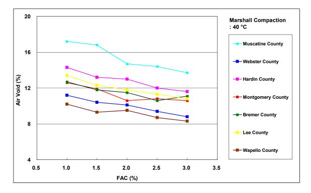
Figure 7-8. Air void of Marshall hammer compacted specimens against FAC (40°C)
