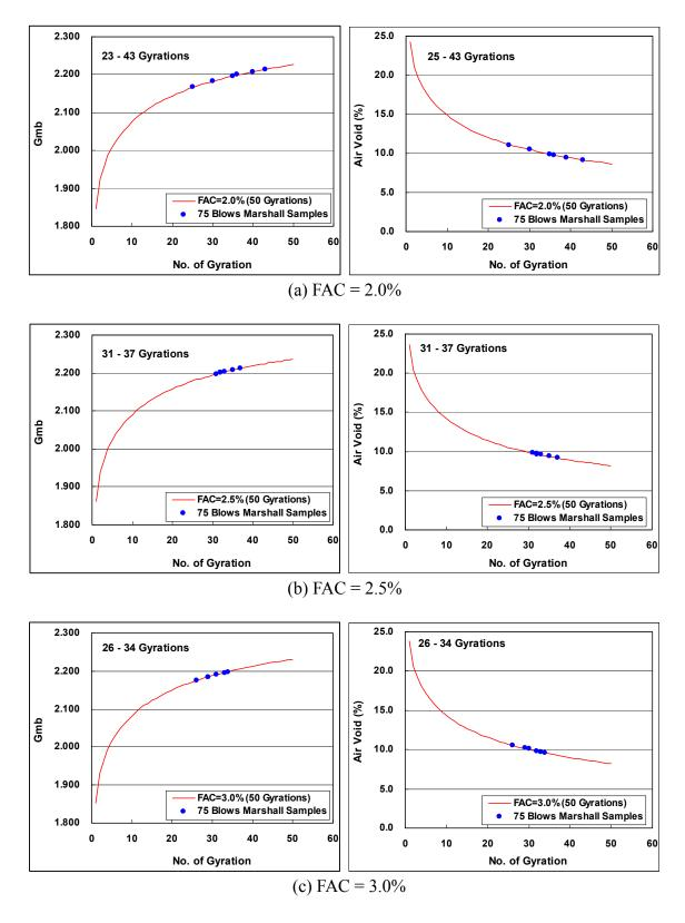
Figure 3-11. Correlation of G<sub>mb</sub> and air void between gyratory and Marshall compacted foamed asphalt specimens (US-20 Highway)
