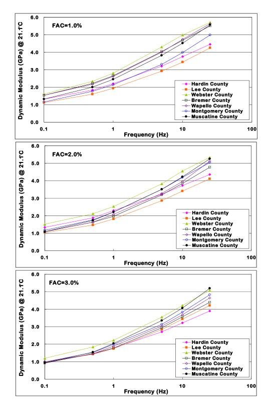
Figure 8-5. Plots of dynamic moduli against six loading frequencies for three foamed asphalt contents at 21.1°C
