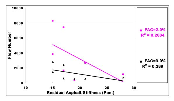
Figure 8-28. Correlation between flow number and residual asphalt stiffness
