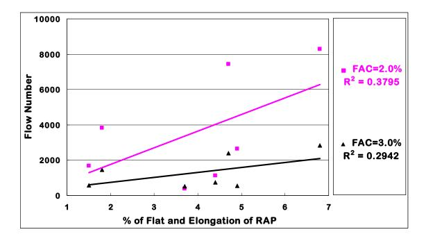
Figure 8-30. Correlation between flow number and % of flat and elongation
