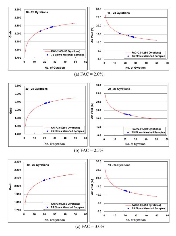
Figure 3-12. Correlation of G<sub>mb</sub> and air void between gyratory and Marshall compacted foamed asphalt specimens (Delaware County)
