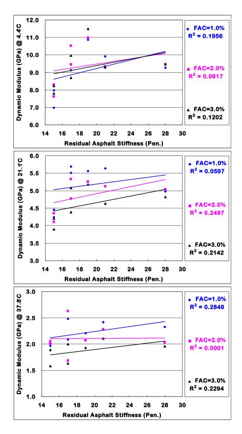
Figure 8-19. Correlation between dynamic moduli and residual asphalt stiffness at three different temperatures
