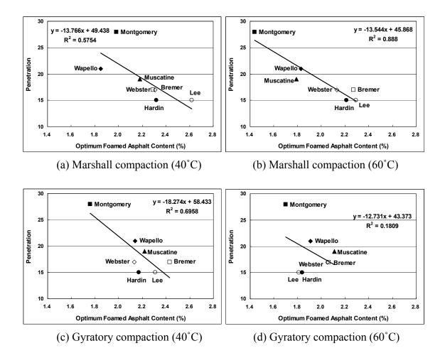
Figure 7-19. Correlations between optimum foamed asphalt content and residual asphalt stiffness
