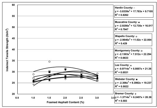
(a) Curing condition: three days at 40°C oven
