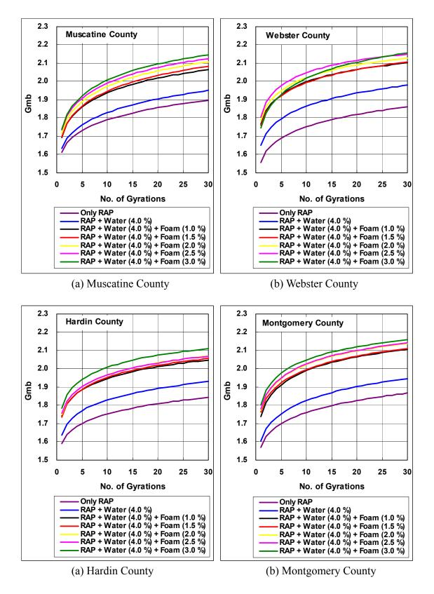
Figure 6-12. Plots of bulk specific gravities against the number of gyrations (1)
