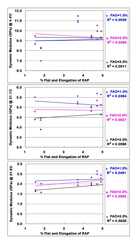
Figure 8-21. Correlation between dynamic moduli and flat & elongation ratio at three different temperatures
