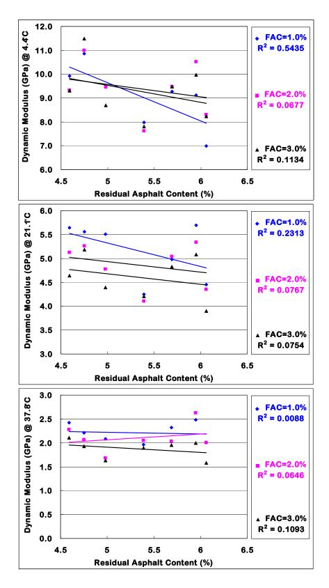
Figure 8-18. Correlation between dynamic moduli and residual asphalt content at three different temperatures
