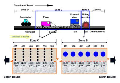
Figure 10-20. Location of collected RAP materials and paved foamed asphalt mixtures in Harrison County project sites
