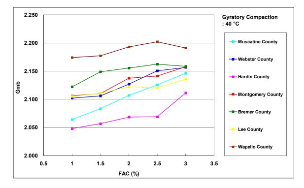
Figure 7-4. G<sub>mb</sub> of gyratory compacted specimens against FAC (40°C)
