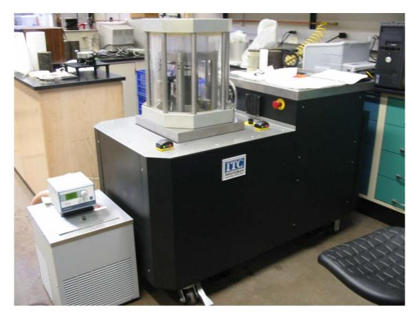
Figure 8-2. Simple performance testing equipment
