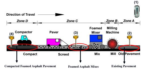
Zone A: Existing Pavement, Zone B: Milling Process, Zone C: Mixing and Paving Process Zone D: Compaction Process
