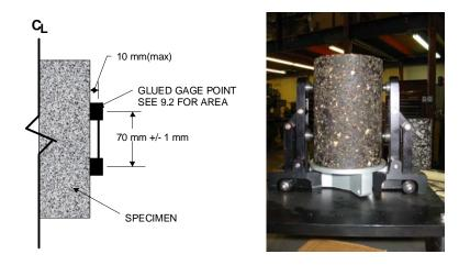
Figure 8-3. Glued magnetic gauge points placed on both sides SPT specimen
