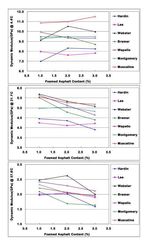
Figure 8-8. Dynamic moduli against three foamed asphalt contents at 25Hz
