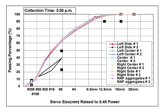
Figure 10-31. Gradations of burned foamed asphalt mixture aggregates collected at 3:30 p.m. across the lane
