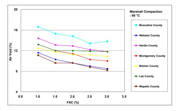
Figure 7-10. Air void of Marshall hammer compacted specimens against FAC (60°C)
