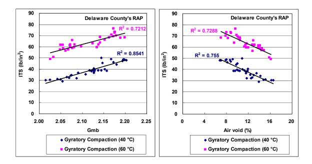
Figure 3-16. Plots of correlation between ITS and G<sub>mb</sub> (and air void) at two different curing temperatures (Delaware County)
