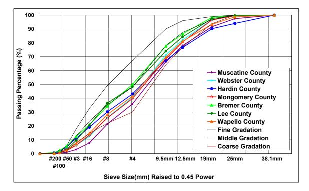
Figure 5-3. Gradation plots of seven different RAP materials
