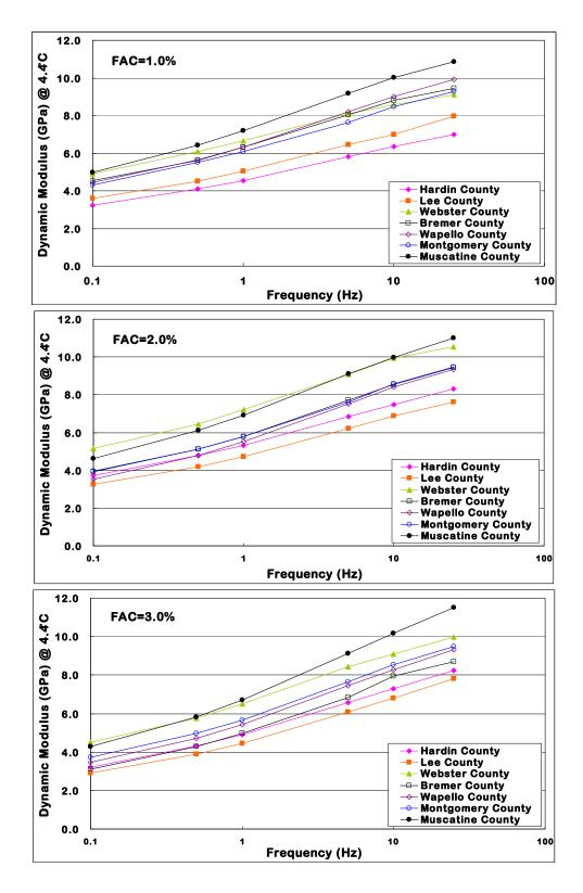
Figure 8-4. Plots of dynamic moduli against six loading frequencies for three foamed asphalt contents at 4.4°C
