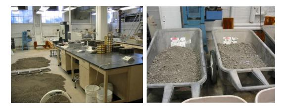
Figure 10-23. Drying process of the RAP materials at the laboratory
