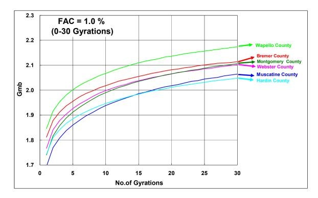
Figure 6-7. Plots of  $G_{mb}$  of RAP materials with 1.0% FAC against the number of gyrations up to 30
