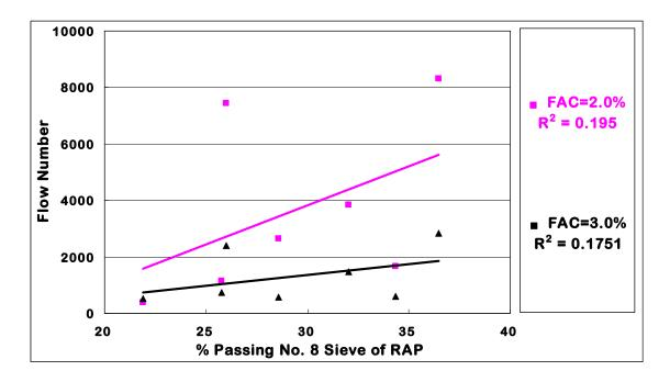
Figure 8-29. Correlation between flow number and % passing No.8 sieve
