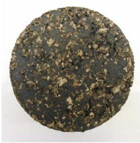
(a) Gyratory compacted specimens (40°C)
