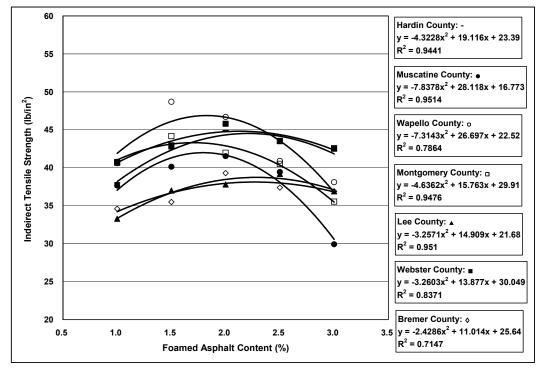
(b) Curing condition: two days at 60°C oven
