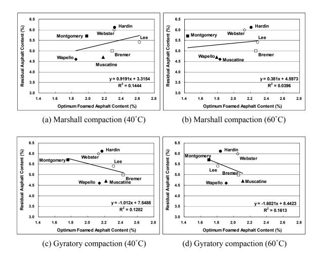
Figure 7-21. Correlations between optimum FAC content and residual asphalt content
