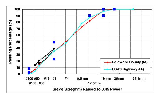
Figure 3-2. RAP gradations of two different RAP materials
