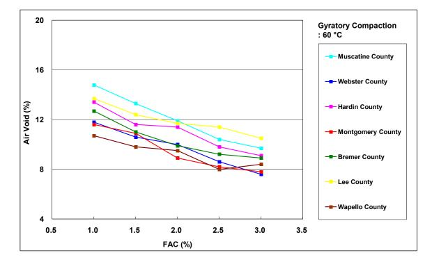
Figure 7-11. Air void of gyratory compacted specimens against FAC (60°C)
