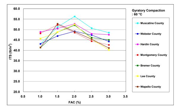
Figure 7-16. ITS of gyratory compacted foamed asphalt specimens (60°C)
