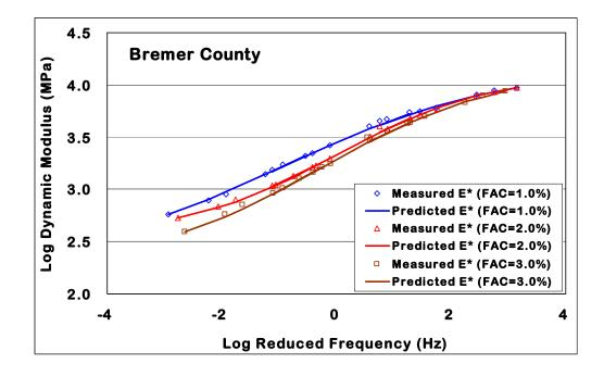
Figure 8-13. Mater curves at three FAC's from Bremer County
