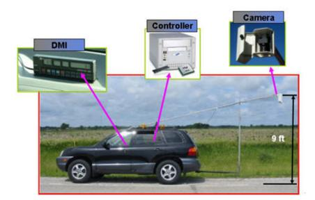
Figure 9-1. Picture of automated image collection system
