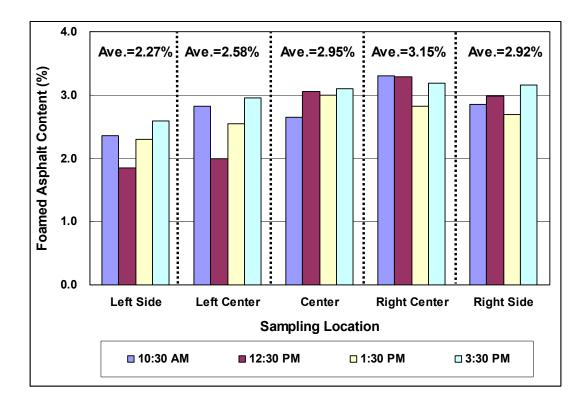
Figure 10-33. Foamed asphalt contents against five different spots across lane
