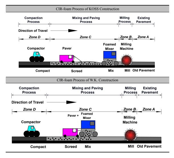
Figure 10-9. Schematic diagram of the CIR-foam process
