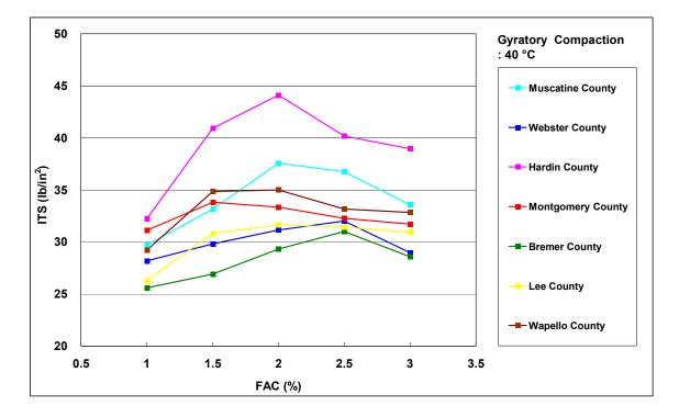
Figure 7-14. ITS of gyratory compacted foamed asphalt specimens (40°C)
