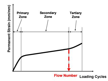
Figure 8-22. Permanent deformation behavior against loading cycles
