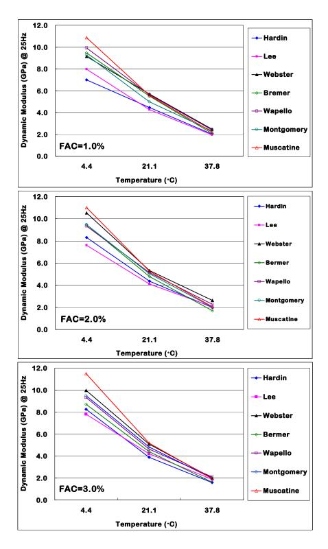
Figure 8-7. Dynamic moduli against three temperatures at 25Hz
