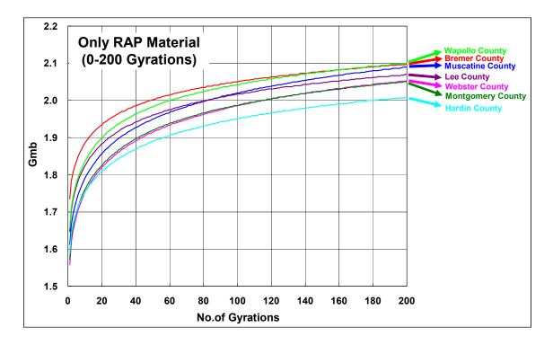
Figure 6-3. Plots of G<sub>mb</sub> of RAP materials against the number of gyrations up to 200
