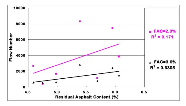
Figure 8-27. Correlation between flow number and residual asphalt content
