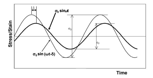
Figure 8-1. Testing components of the dynamic modulus
