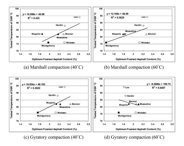
Figure 7-20. Correlations between optimum foamed asphalt content and testing temperature of DSR
