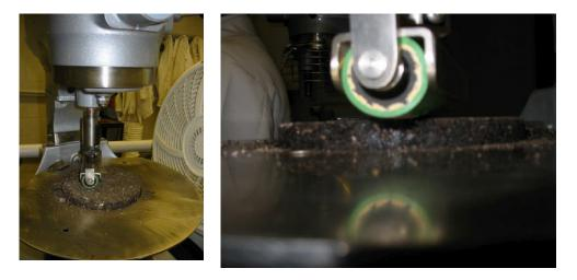
Figure 8-31. Pictures of raveling test equipment
