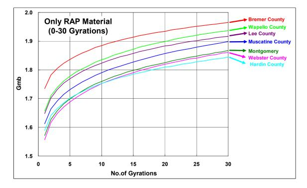
Figure 6-4. Plots of G<sub>mb</sub> of RAP materials against the number of gyrations up to 30
