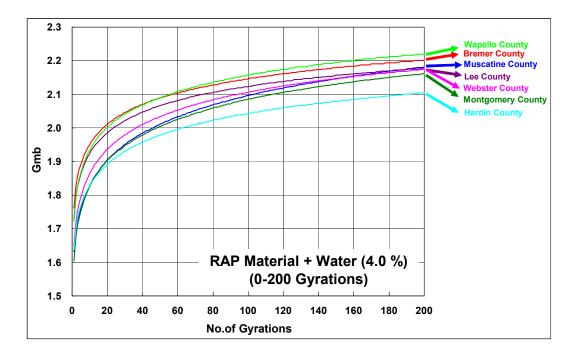
Figure 6-5. Plots of G<sub>mb</sub> of RAP materials with 4.0% water against the number of gyrations up to 200
