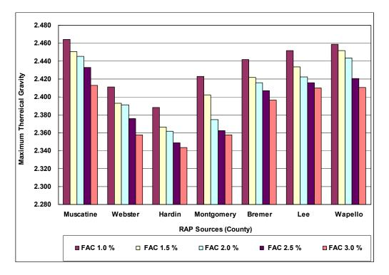
Figure 7-7. Plots of theoretical maximum specific gravities
