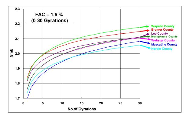
Figure 6-8. Plots of  $G_{mb}$  of RAP materials with 1.5% FAC against the number of gyrations up to 30
