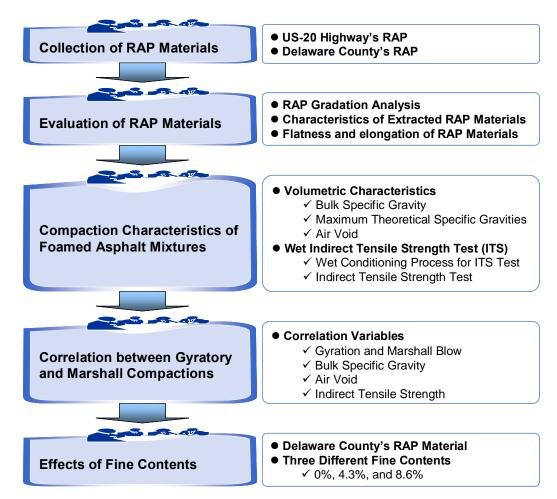
Figure 3-1. Test flowchart and parameters of pilot study
