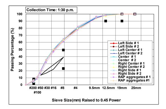
Figure 10-30. Gradations of burned foamed asphalt mixture aggregates collected at 1:30 p.m. across the lane
