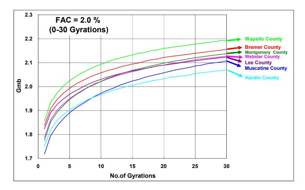
Figure 6-9. Plots of  $G_{mb}$  of RAP materials with 2.0% FAC against the number of gyrations up to 30
