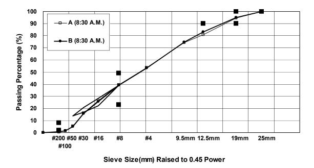
Figure 10-27. Gradation plots of RAP materials passing 25 mm colleted at one time period in Johnson County project
