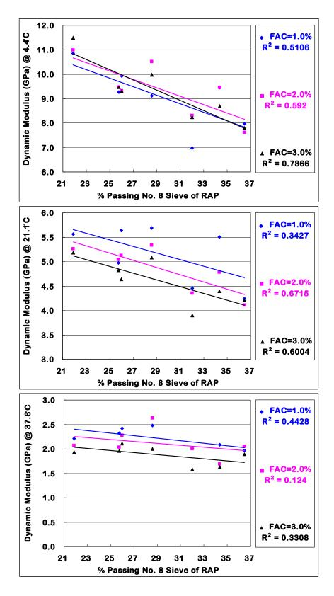
Figure 8-20. Correlation between dynamic moduli and amount of fine RAP materials passing No. 8 sieve at three different temperatures
