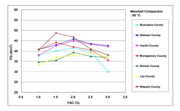
Figure 7-15. ITS of Marshall compacted foamed asphalt specimens (60°C)
