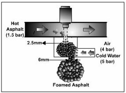
(b) Production of foamed asphalt in the expansion chamber
