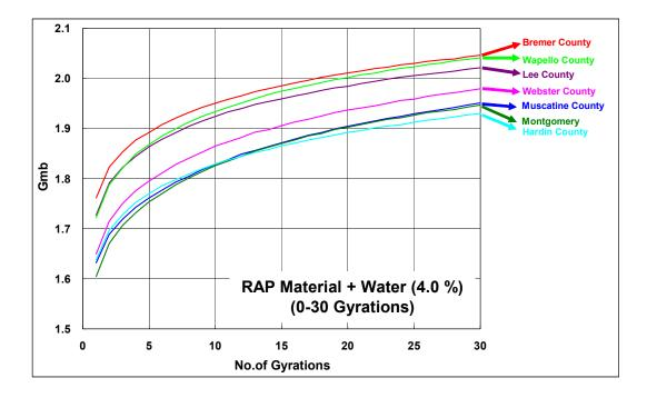
Figure 6-6. Plots of  $G_{mb}$  of RAP materials with 4.0% water against the number of gyrations up to 30
