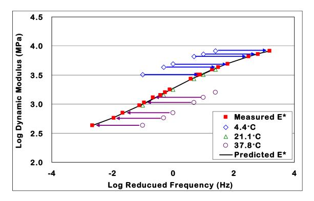
Figure 8-9. Construction of master curve
