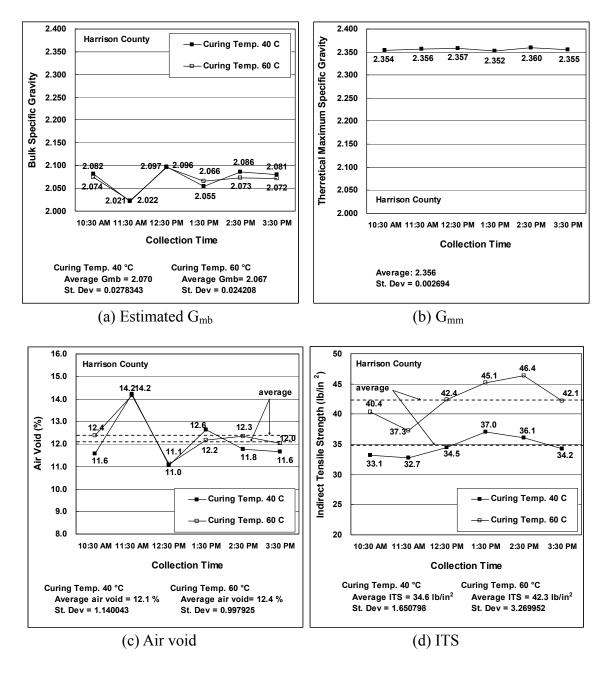
Figure 10-35. Volumetric characteristics and ITS of foamed asphalt mixture collected from Harrison County project
