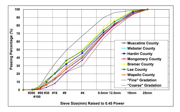
Figure 5-4. Gradation plots of seven different RAP materials passing 25mm sieve
