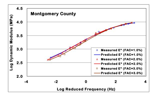
Figure 8-15. Mater curves at three FAC from Montgomery County
