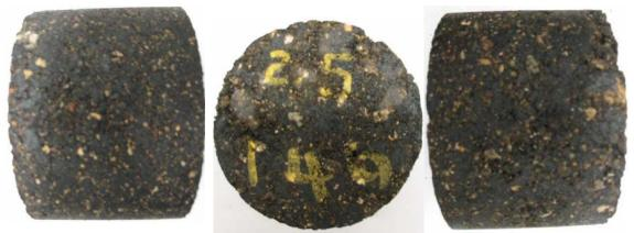
(c) Foamed asphalt specimens with 2.5% FAC and 4.0% water
