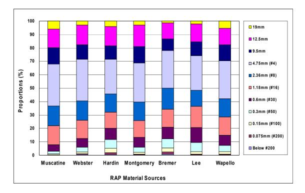
Figure 5-5. Cumulated gradation bar charts of seven different RAP materials passing 25mm sieve
