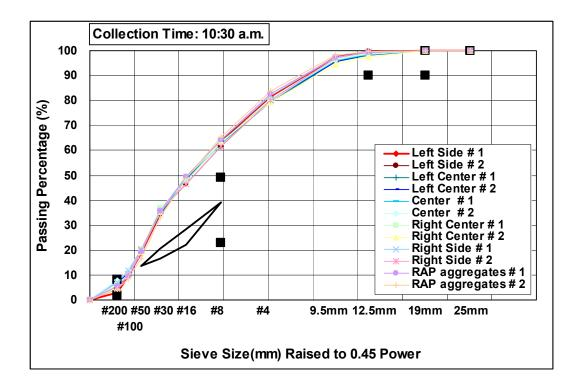
Figure 10-28. Gradations of burned foamed asphalt mixture aggregates collected at 10:30 a.m. across the lane
