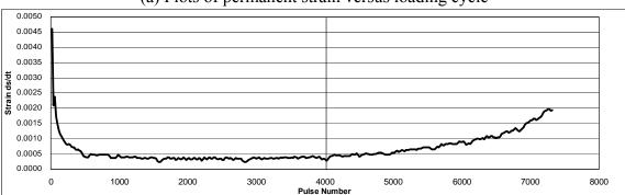
(b) Rate of change in permanent strain versus loading cycle
