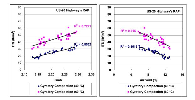
Figure 3-15. Plots of correlation between ITS and G<sub>mb</sub> (and air void) of specimens at two different curing temperatures (US Highway)
