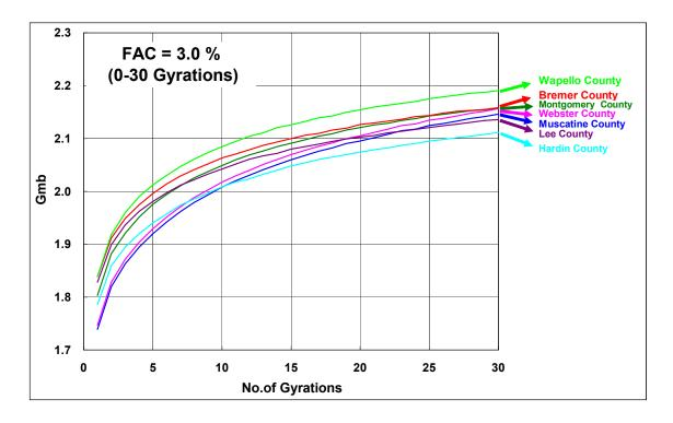
Figure 6-11. Plots of  $G_{mb}$  of RAP materials with 3.0% FAC against the number of gyrations up to 30
