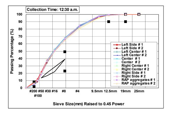
Figure 10-29. Gradations of burned foamed asphalt mixture aggregates collected at 12:30 p.m. across the lane
