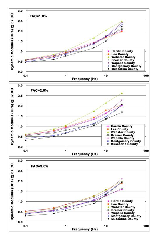
Figure 8-6. Plots of dynamic modulus value against six loading frequencies for three foamed asphalt contents at 37.8°C
