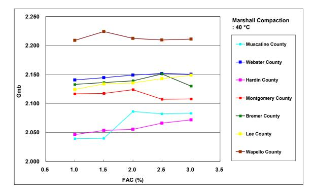
Figure 7-3. G<sub>mb</sub> of Marshall hammer compacted specimens against FAC (40°C)
