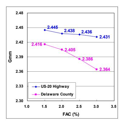
Figure 3-7. Plot of theoretical maximum specific gravity against foamed asphalt contents for two different RAP sources
