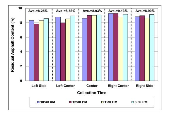
Figure 10-32. Residual asphalt contents of foamed asphalt mixtures across the lane
