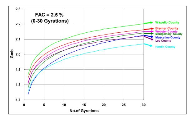
Figure 6-10. Plots of  $G_{mb}$  of RAP materials with 2.5% FAC against the number of gyrations up to 30
