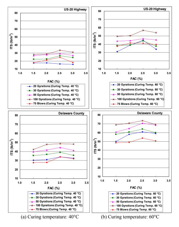
Figure 3-10. Plots of indirect tensile strength against FAC at five different levels of compaction
