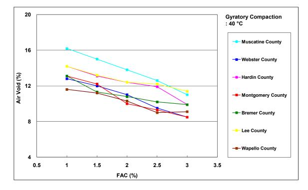
Figure 7-9. Air void of gyratory compacted specimens against FAC (40°C)
