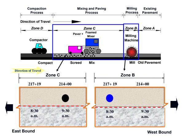
Figure 10-22. Locations of collected RAP materials and foamed asphalt mixtures in Johnson County project sites
