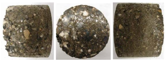
(a) RAP specimens without foamed asphalt and water
