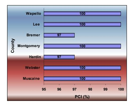
Figure 9-16. Comparison of PCI from distress data at seven CIR project sites
