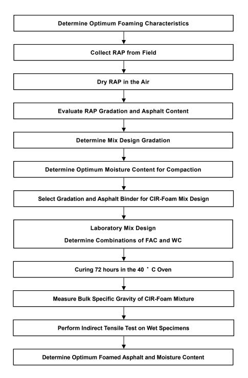
Figure 2-2. Developed new laboratory mix design procedure of CIR-foam
