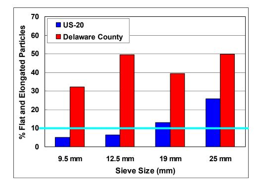
Figure 3-4. Comparison of % flat and elongated particles at two different RAP sources
