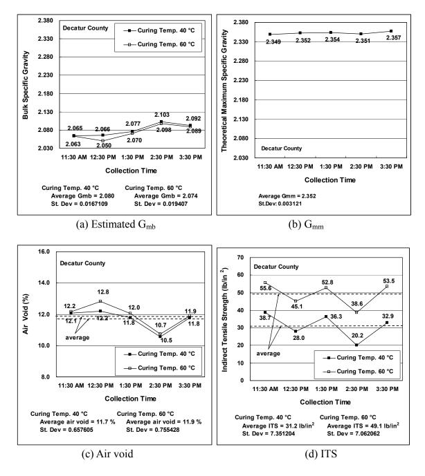
Figure 10-34. Volumetric characteristics and ITS of foamed asphalt mixture collected from Decatur County project
