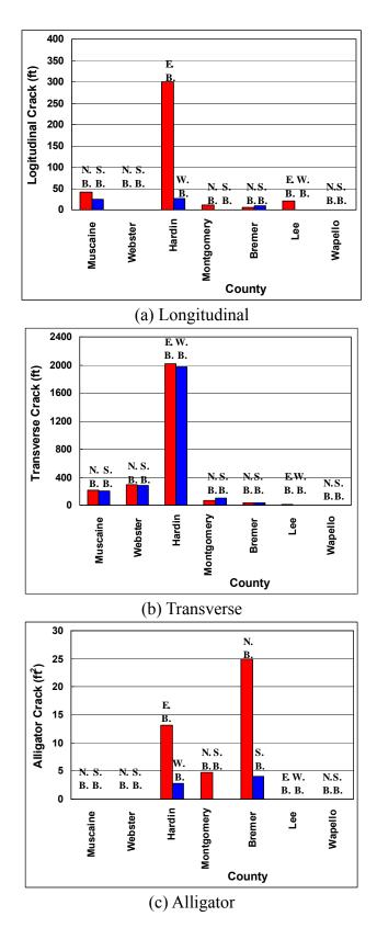
Figure 9-3. Longitudinal, transverse, and alligator cracks measured from overlaid HMA pavement on CIR layer
