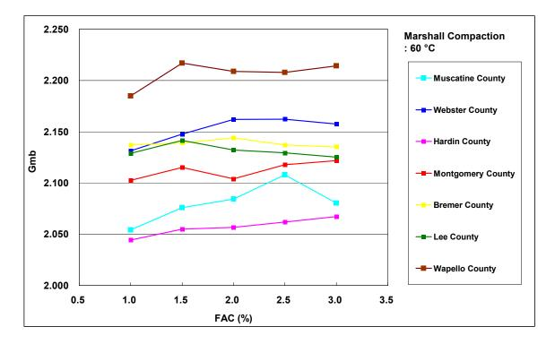
Figure 7-5. G<sub>mb</sub> of Marshall hammer compacted specimens against FAC (60°C)
