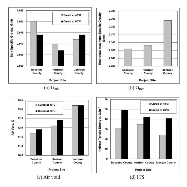
Figure 10-36. Comparisons of volumetric characteristics and ITS of foamed asphalt mixture collected from three CIR-foam project sites
