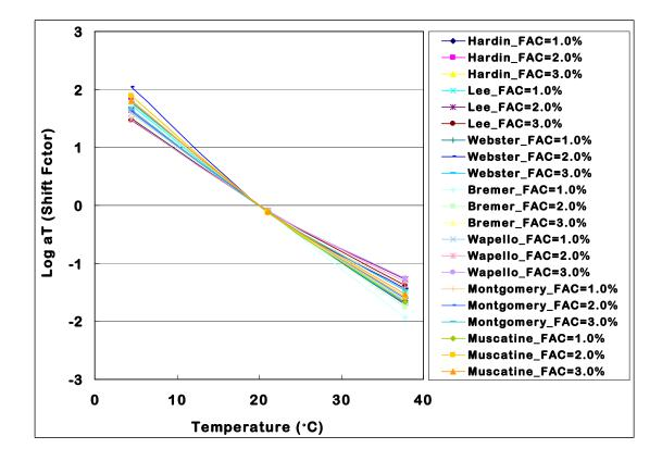
Figure 8-17. Shift factors against three temperatures
