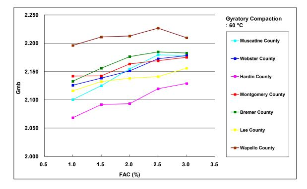
Figure 7-6. G<sub>mb</sub> of gyratory compacted specimens against FAC (60°C)
