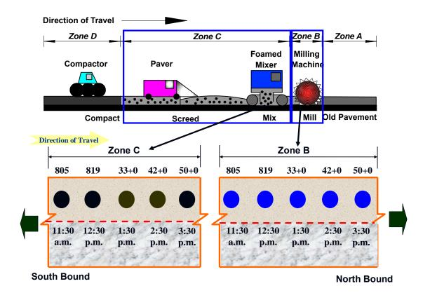
Figure 10-18. Location of collected RAP materials and foamed asphalt mixtures in Decatur County project sites
