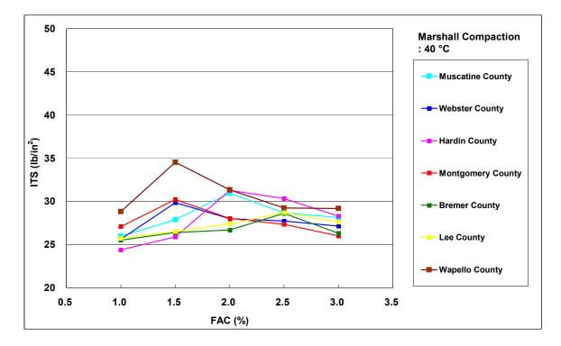
Figure 7-13. ITS of Marshall compacted foamed asphalt specimens (40°C)
