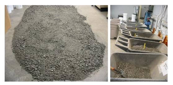
Figure 5-1. Drying process of the RAP materials at the laboratory
