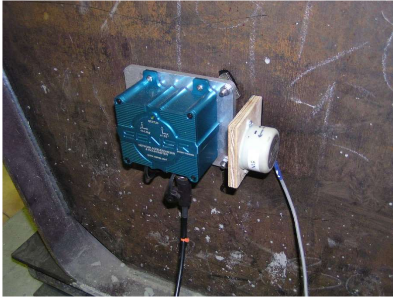
Figure 2. Photograph of SENSr Sensor and Conventional Tilt Sensor
