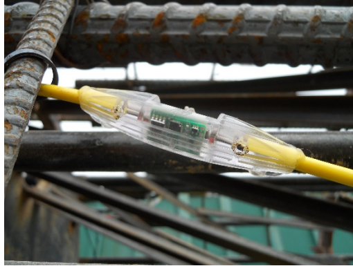
Figure 2: Close up of encapsulated temperature sensor and circuit board in PDI Thermal Wire® cable system.
