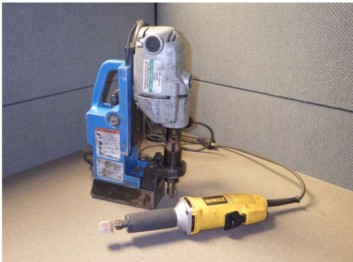
Figure 1 – typical magnetic drill press and die grinder used for crack arrest holes
