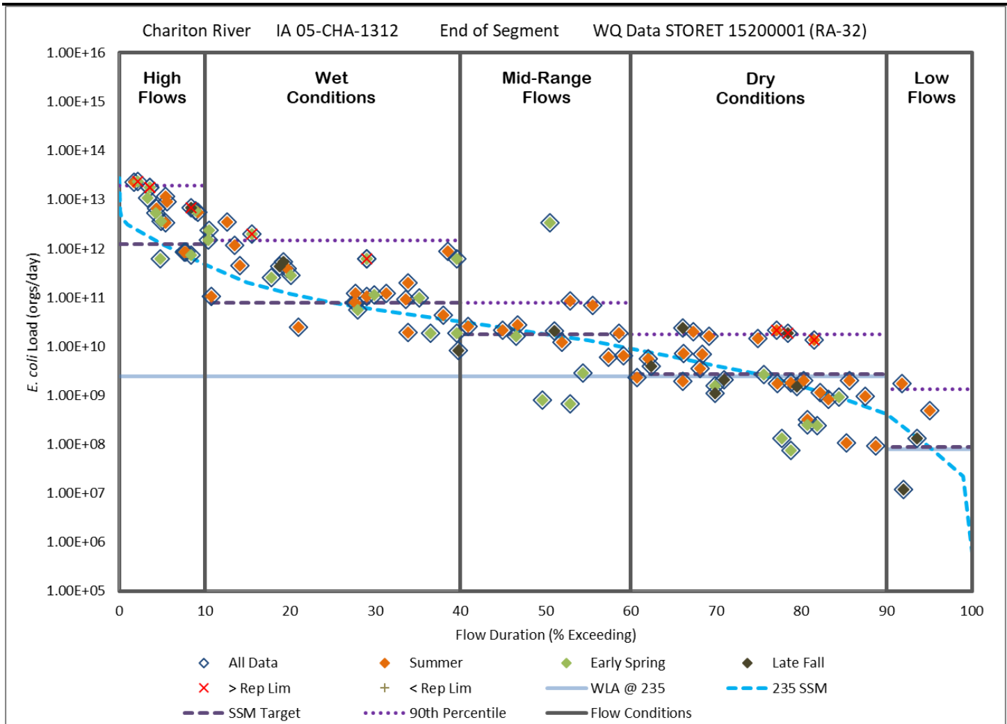
Figure 4.8. Load Duration Curve based on the SSM for IA 05-CHA-1312.
