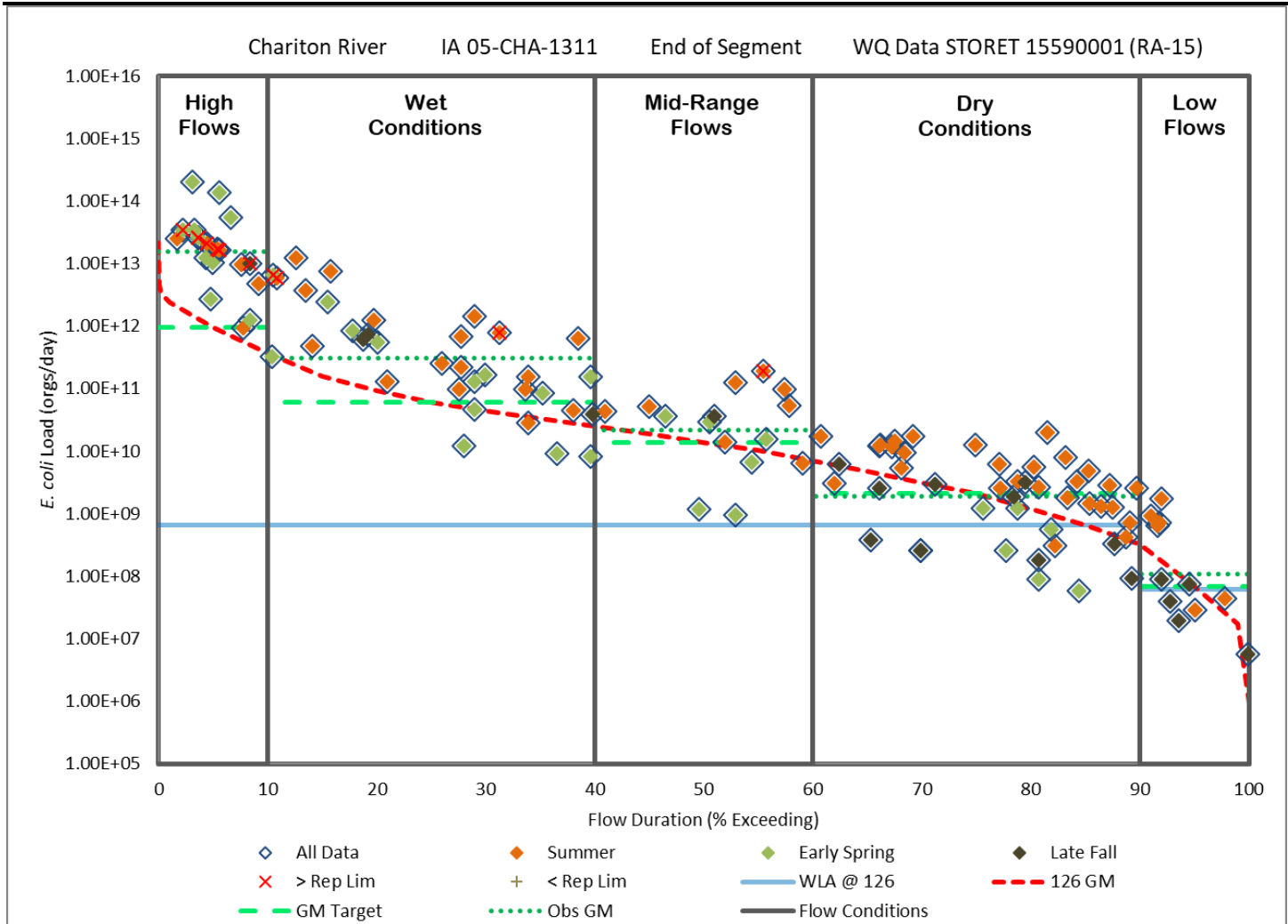
Figure 4.7. Load Duration Curve based on the GM for IA 05-CHA-1311.
