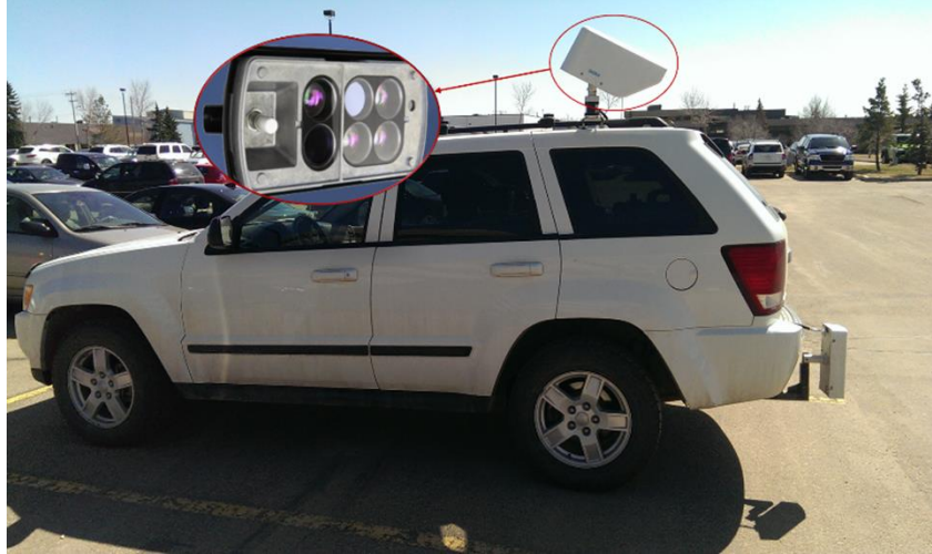
Figure 1.2. Mobile RWIS unit equipped with spectral road surface temperature sensor
