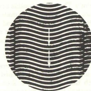
Figure 13c. Magnified frontal view of the Hydrasieve showing the ripple conformation to windrow the solids as they traverse the front of the screen.
