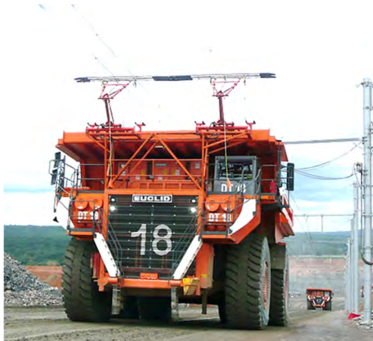
FIGURE 2 Example of channelized loading on a trolley assist ramp (reproduced with permission http://www.metalsnews.com ).
