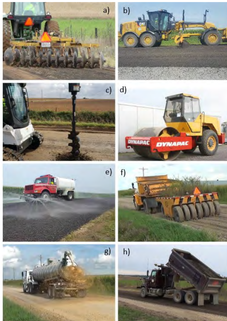
FIGURE 1 Equipment used for mechanically stabilized sections: (a) disk plow harrow; (b) motor grader; (c) power auger; (d) vibratory compactor; (e) water truck; (f) rubber tire roller; (g) self-unloading tanker trailer spraying clay slurry; and (h) dump truck.
