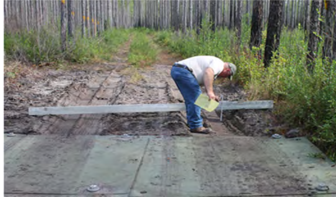
FIGURE 3 Rut depth measurement of control section, Apalachicola National Forest.
