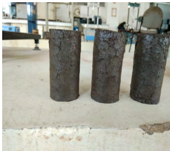
FIGURE 6 UCS testing of BC soil sample after testing.
