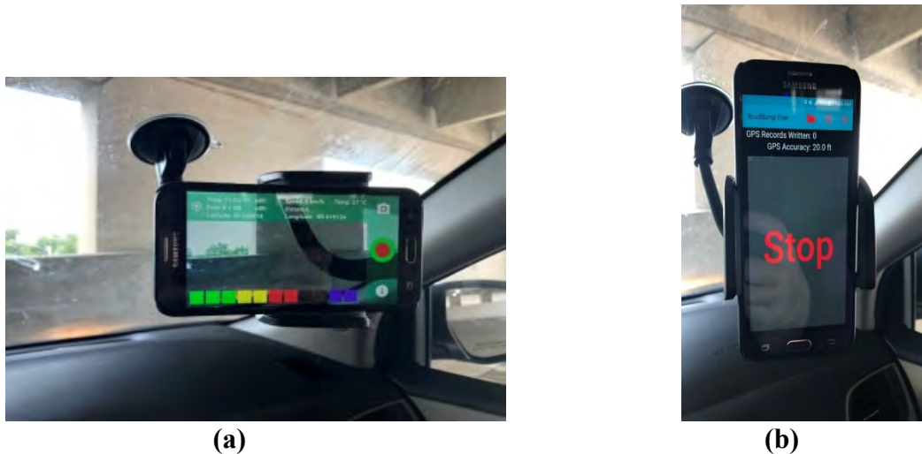
FIGURE 3 Cell phone apps used in this study: (a) Roadroid app on cell phone and (b) RoadBump app on cell phone
