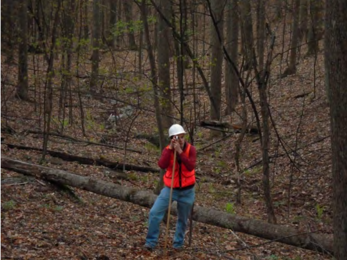
FIGURE 2 Students use simple hand levels or clinometers for grade-line installation.
