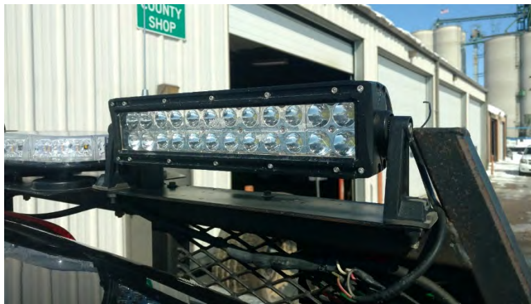
FIGURE 1 LED light to illuminate the sign and create the headlight effect used for nighttime inspections.
