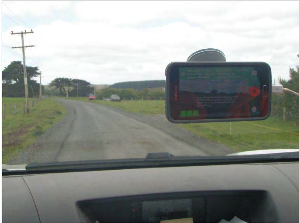
FIGURE 4 Roadroid phone as mounted for surveys.
