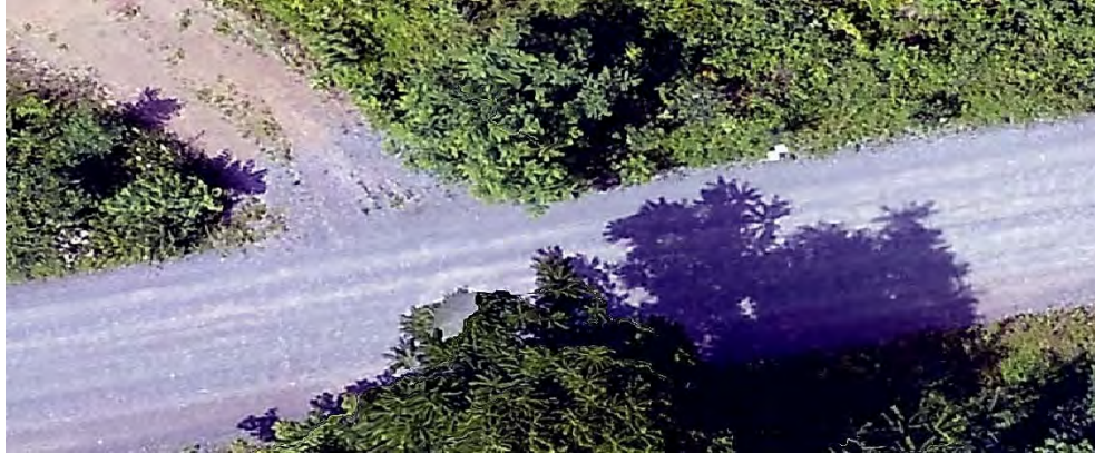
FIGURE 1 Photo showing edge of road vegetation shading the road surface. Note the high-quality image resolution of 2 to 3 cm per pixel.
