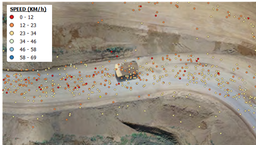
FIGURE 10 Example of events collected from the truck fleet by the dispatch management system.
