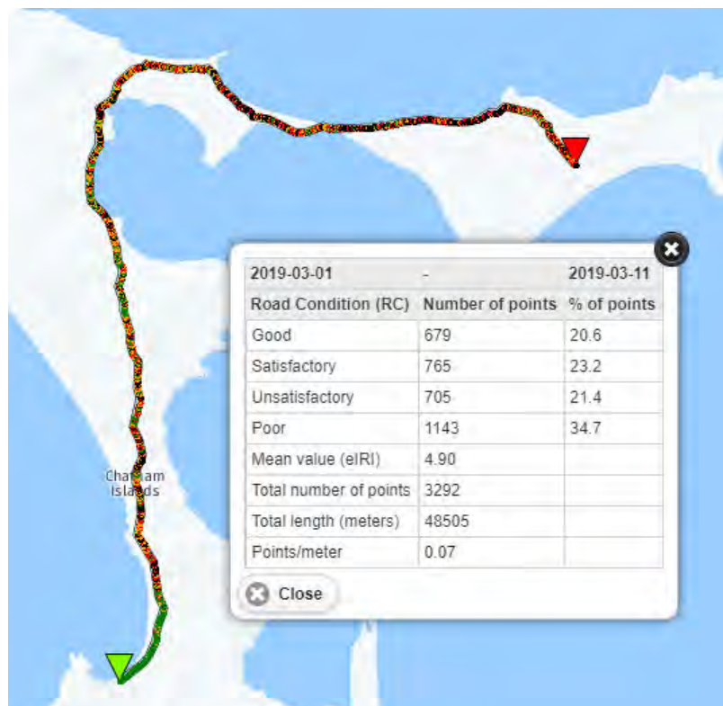
FIGURE 5 Condition analysis calculated directly from Roadroid server.
