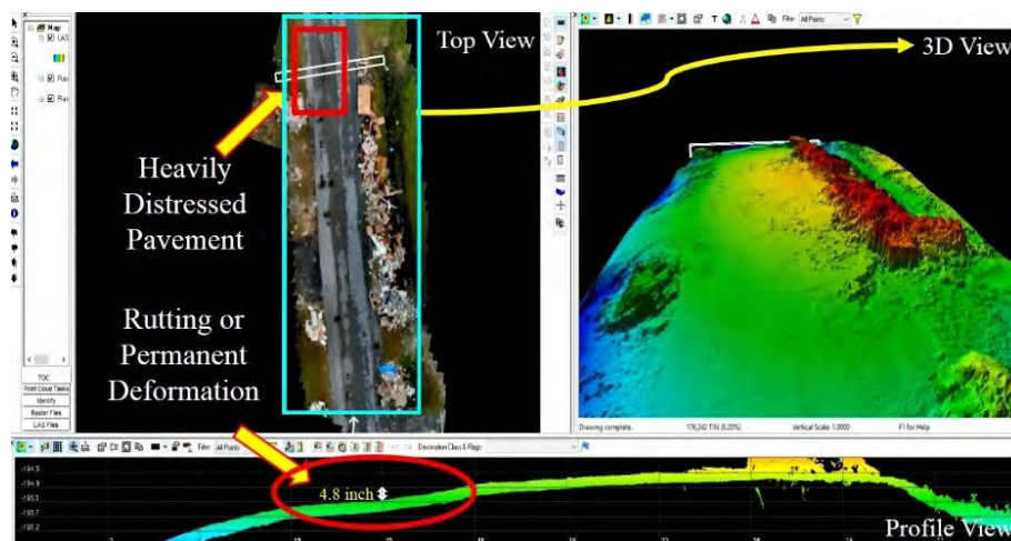
FIGURE 4 UAV-CRP technology data identifying rutting of pavement section immediately after Hurricane Harvey.
