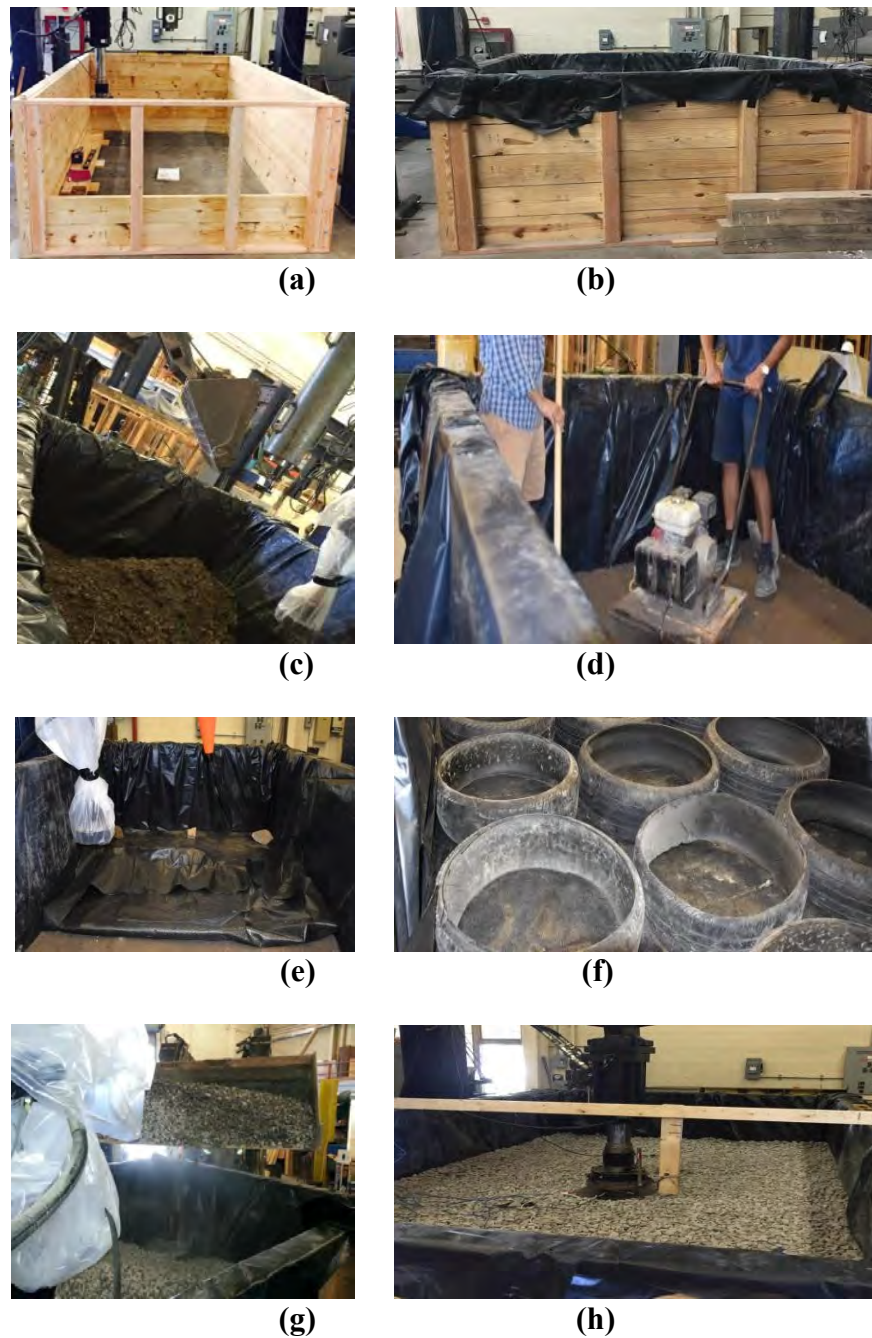
FIGURE 1 Bin construction: (a) frame construction; (b) polyethylene sheet-lined wooden bin; (c) soil placement; (d) soil compaction, three 150-mm lifts; (e) placement of separation woven geotextile fabric on compacted soil; (f) placement of TDGCs over separation fabric; (g) placement of AASHTO #57 aggregate as infill for the TDGCs; and (h) aggregates placed 50 mm above TDGC top surface and ready for testing.
