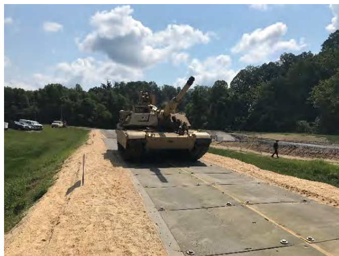
FIGURE 5 M1 Abrams tank on SP test section, ERDC site.
