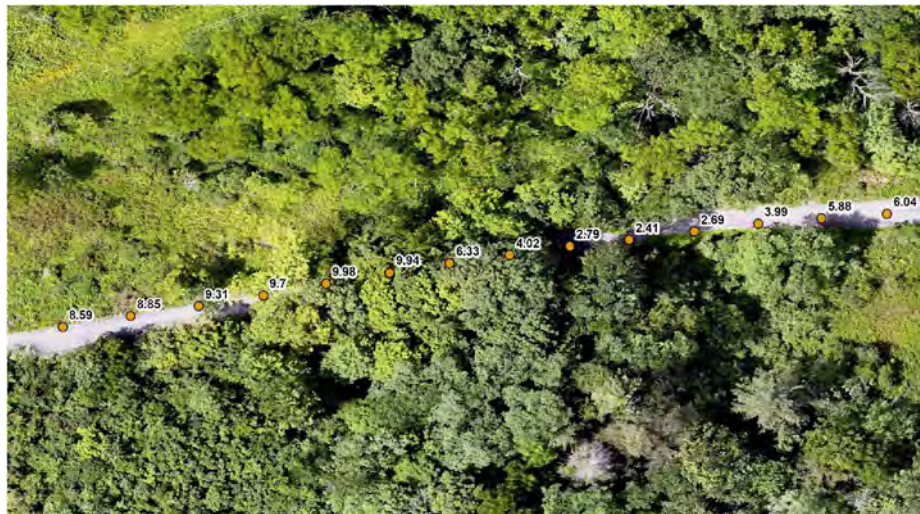
FIGURE 2 Segment of dust-monitoring data points overlain on georeferenced aerial imagery. The monitoring vehicle was traveling from left to right. Note lag in the dust production decrease as vehicle enters road section with full canopy. Dust values in mg/m 3 .
