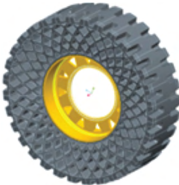
FIGURE 4 Non-pneumatic tire for use on haul trucks and loaders.
