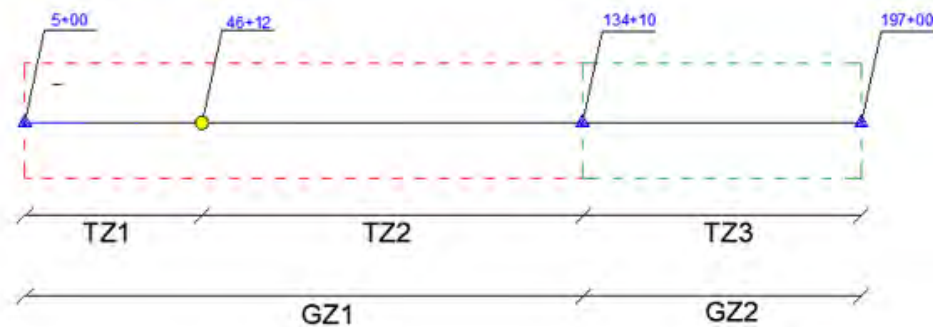
FIGURE 5 Linear representation of the road extension (in Brazilian “estacas” = 20 m). The triangles represent the initial and final point of GZs and the circle represents the division point between TZ 1 and TZ 2.
