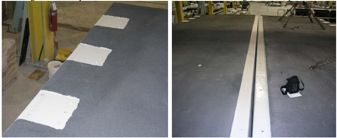
Figure 7. Guardrail and centerline attachment locations
