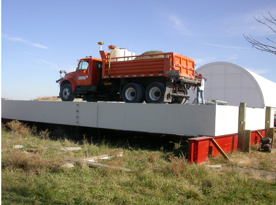
Figure 20. Truck Load Test.
