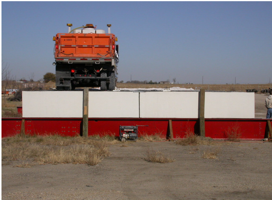
Figure 21. End View Truck Load Test.
