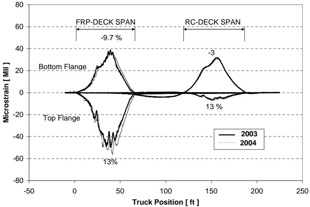
Figure 33. Strain Response Comparison: Girder D – Path Y1
