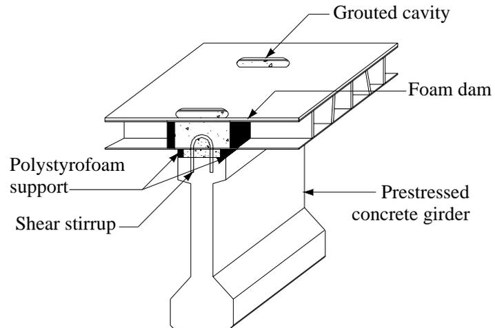
**Figure 11. Composite Action: FRP Panel and Prestressed Concrete Girder**
