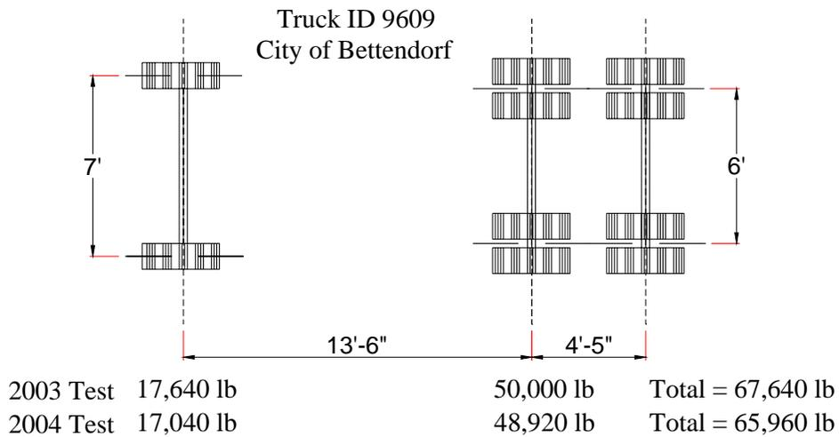
**Figure 23. Geometry and Weight of Test Truck**
