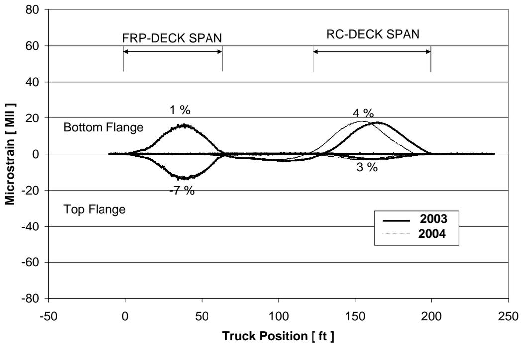
Figure 34. Strain Response Comparison: Girder B – Path Y2
