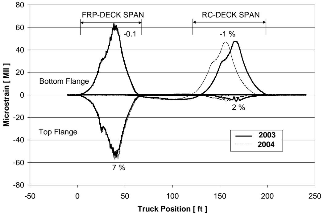
Figure 35. Strain Response Comparison: Girder C – Path Y2
