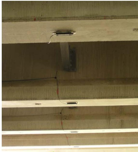
**Figure 24. Overall View of the Long-Term Monitoring System (Peak Strain Sensors)**
