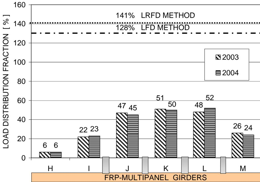
Figure 44. LDF Superposition of Paths Y5 and Y6
