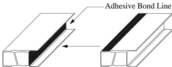
**Figure 1. DuraSpan Deck Panel – Assembly Scheme**
