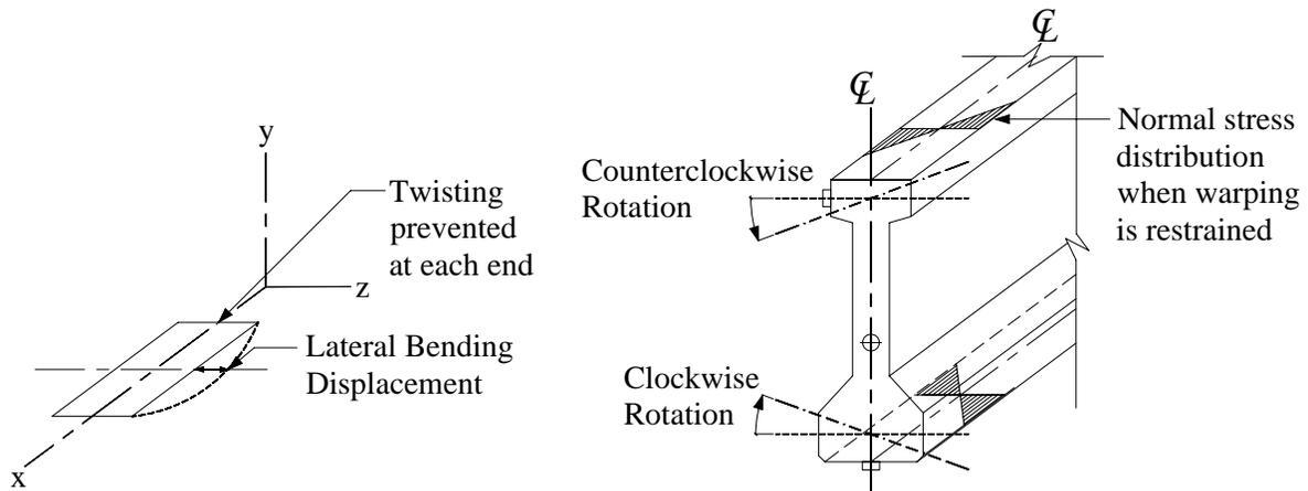
**Figure 50. Effect of Warping Torsion**
