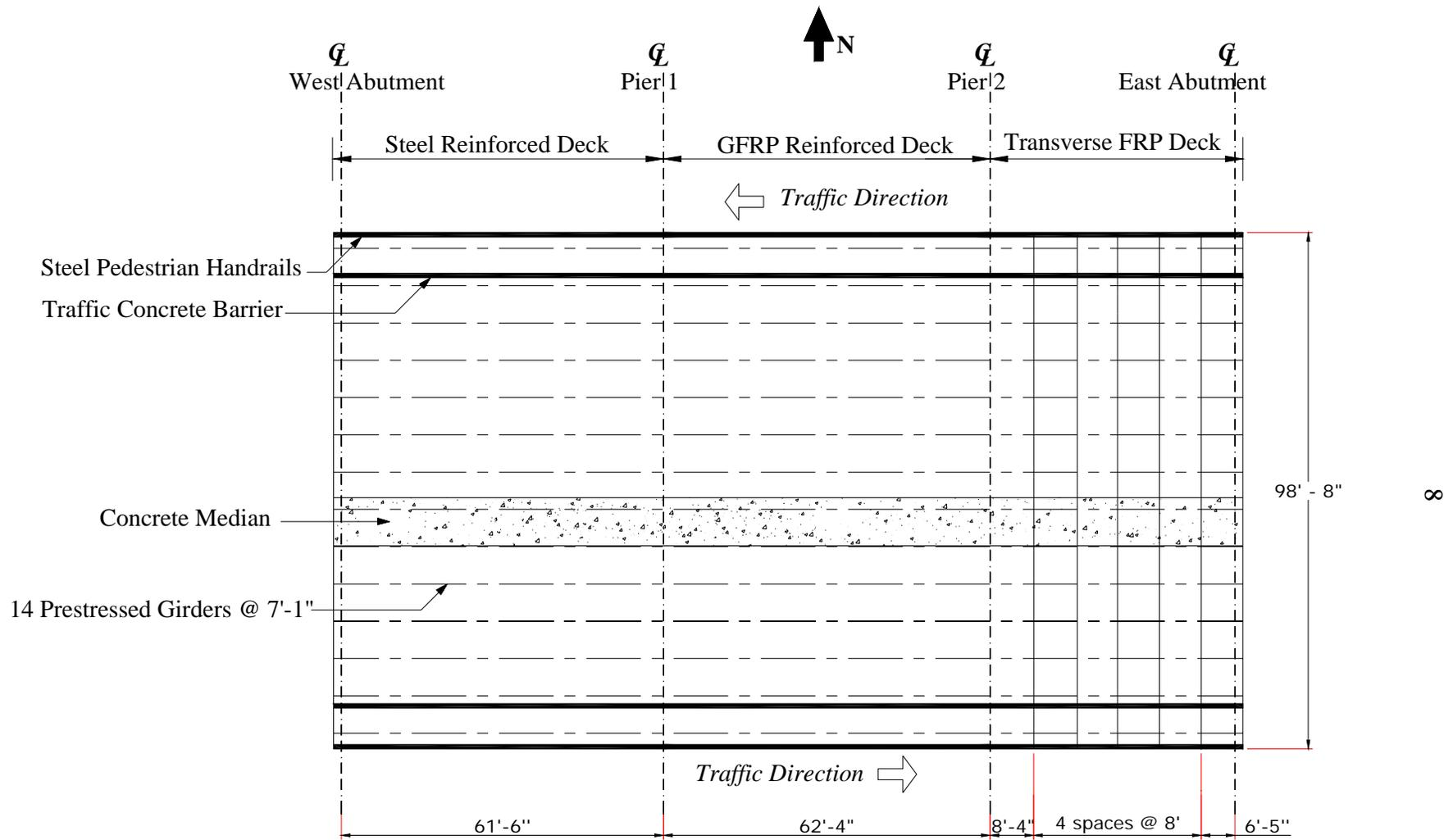
**Figure 4. Plan View of the 53<sup>rd</sup> Avenue Extension Bridge**
