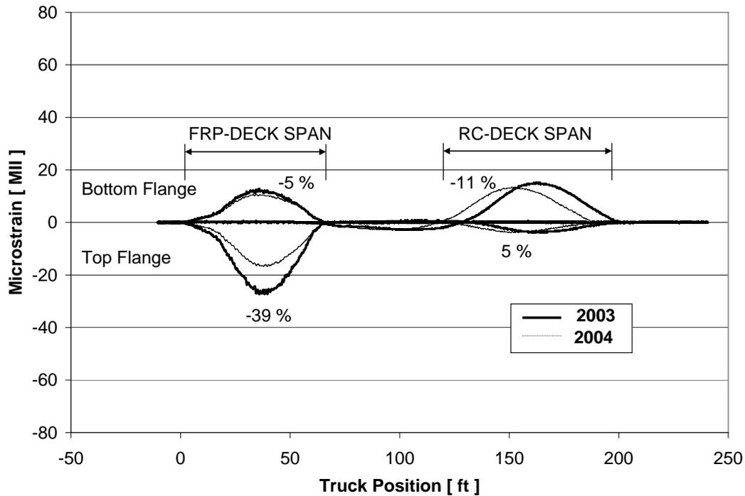
**Figure 37. Strain Response Comparison: Girder E – Path Y2**
