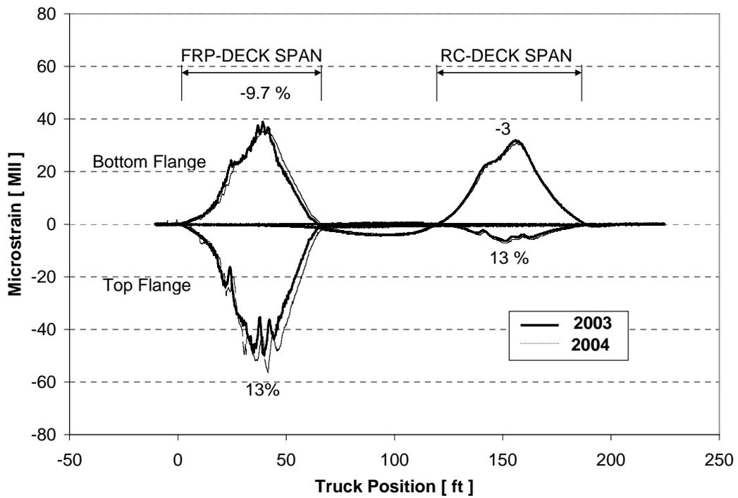
Figure 36. Strain Response Comparison: Girder D – Path Y2
