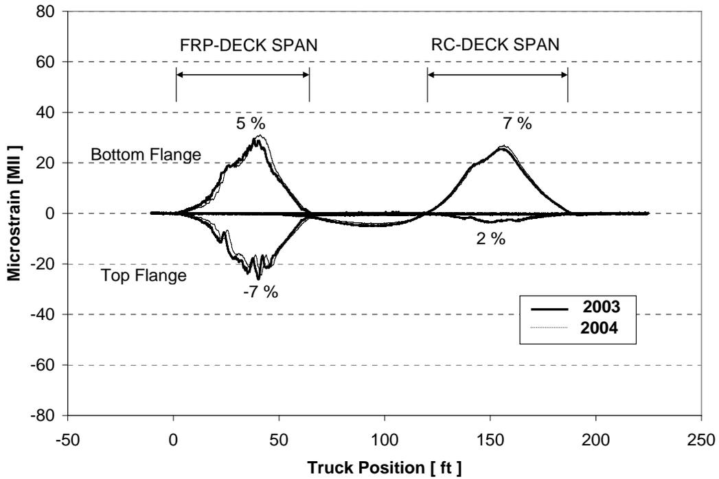
Figure 31. Strain Response Comparison: Girder B – Path Y1
