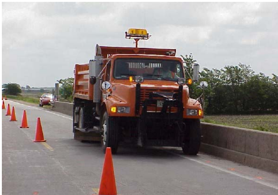
Figure 24. Photograph of typical load test truck.
