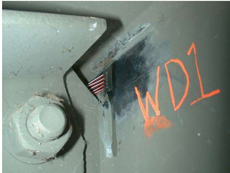
a. Photograph of G1 gradient gage.
