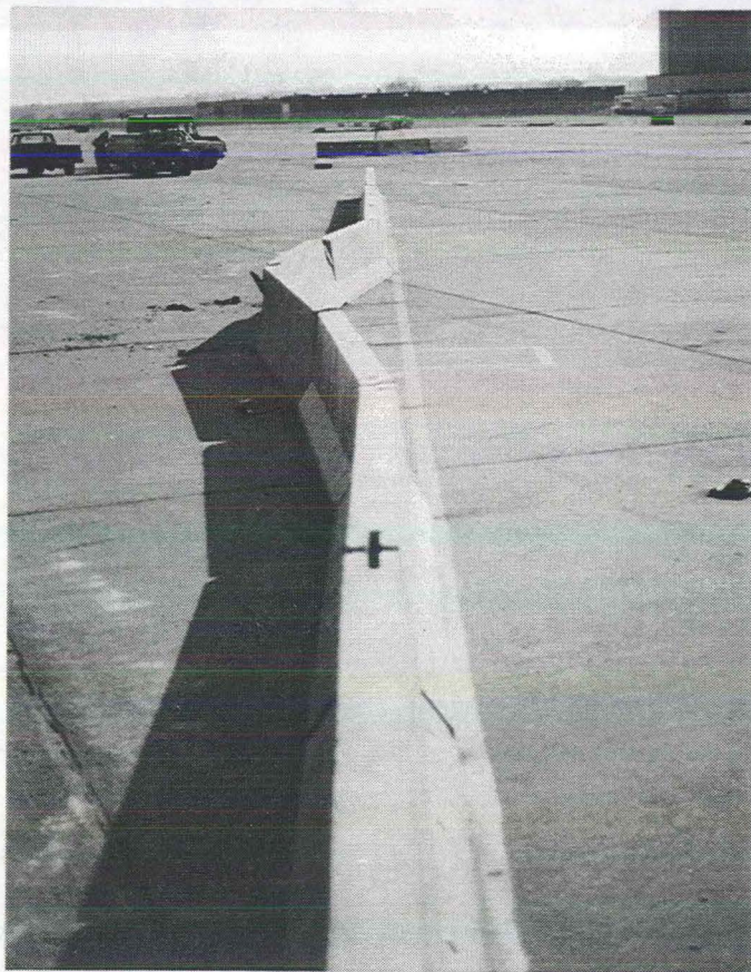
Figure 19. Barrier Damage, Test ITMP-1
