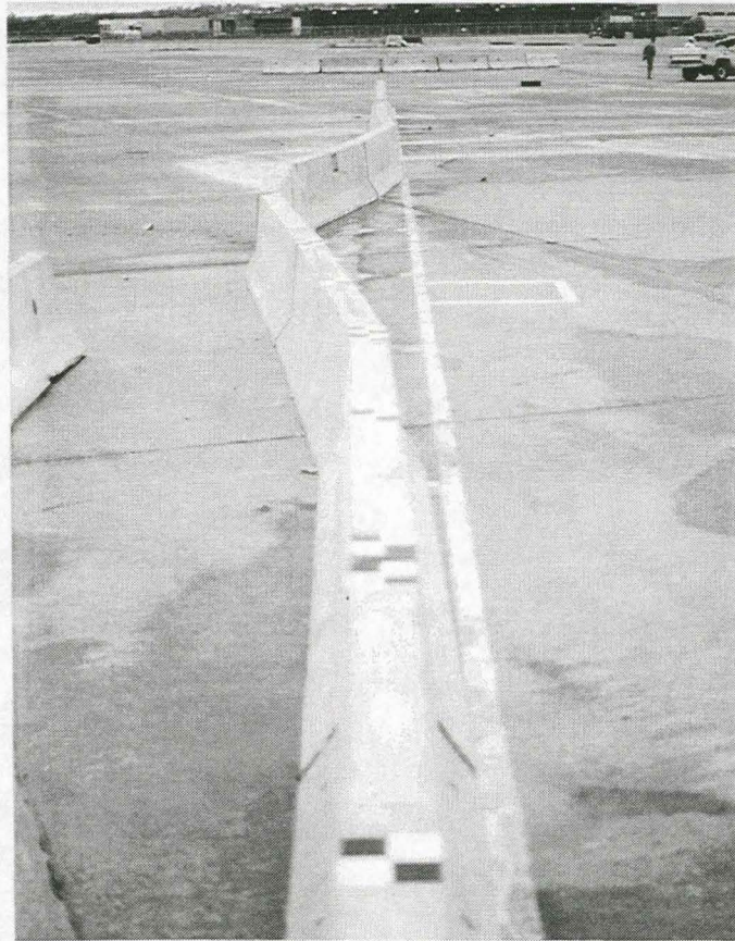
Figure 32. Barrier Damage, Test ITMP-2
