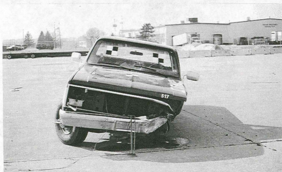
Figure 18. Vehicle Damage, Test ITMP-1
