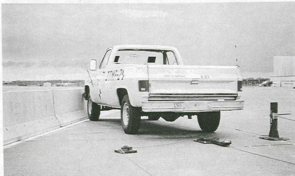
Figure 30. Impact Location, Test ITMP-2
