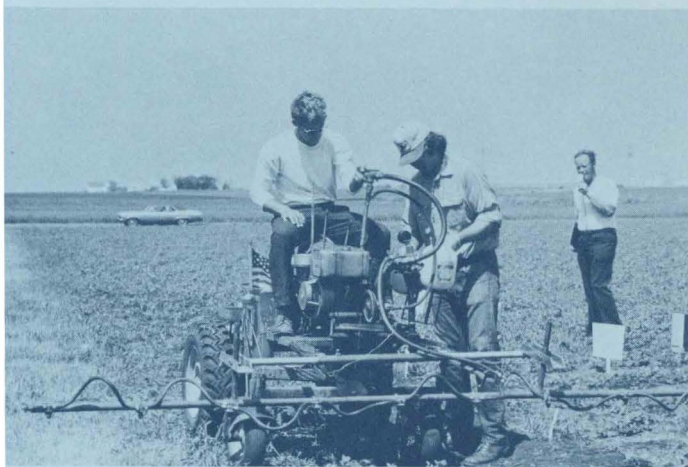
A small, highly maneuverable sprayer is used for accurate placement of chemicals on herbicide-evaluation plots at the Northern Iowa Farm.
