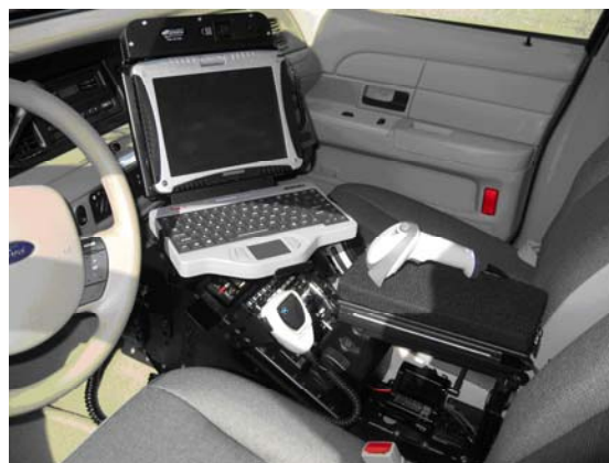
Radio console and computer are standard equipment in an Iowa State Patrol squad car
