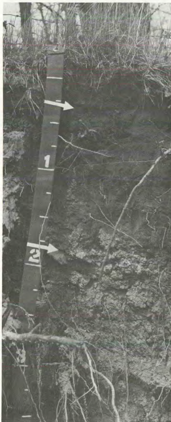
Figure 10.—A profile of Keswick loam formed mostly in Late Sangamon paleosol. The lower part of the profile below a depth of 2 feet is glacial till.
