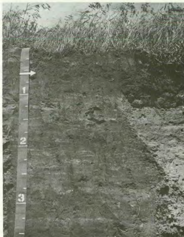
Figure 11.—Profile of Nodaway silt loam. The horizontal strata were deposited by flood water.
