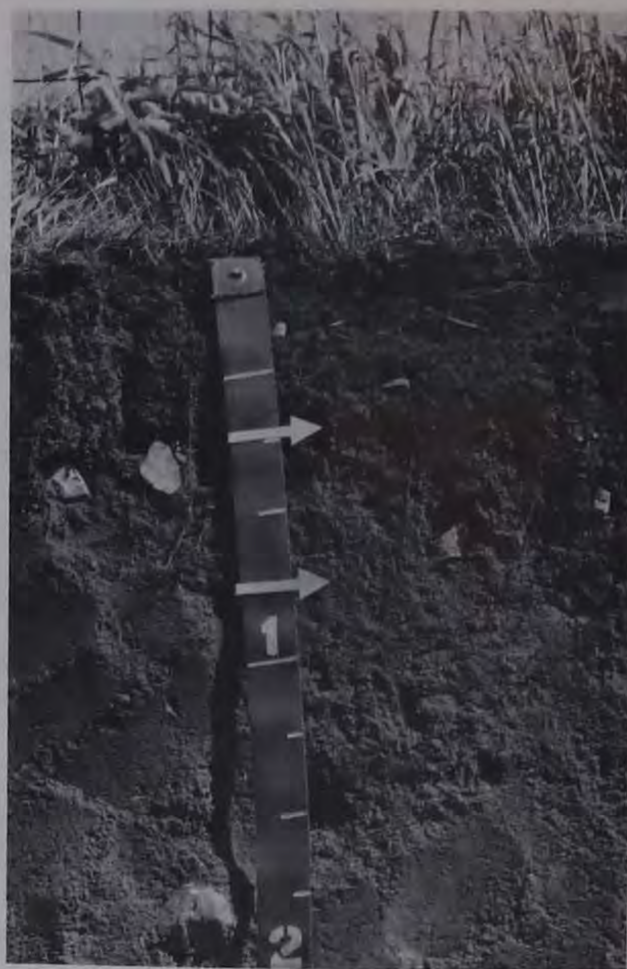
Figure 12.—Profile of Shelby loam. This soil formed in glacial till. Stones and pebbles are common.
