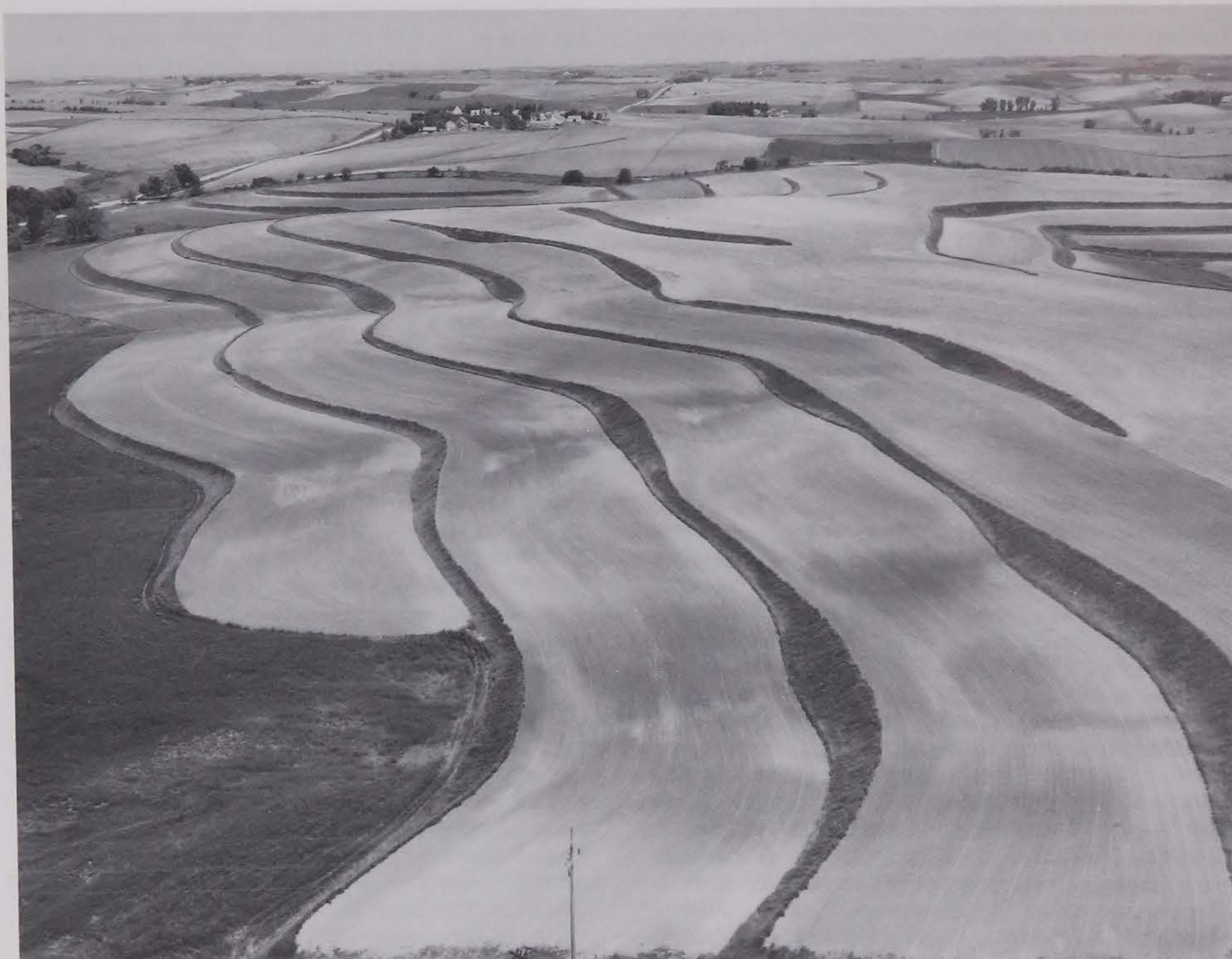
Figure 12.—Erosion on grassed back slope terraces in an area of Monona soils. The small, lighter colored areas are Ida soils.
