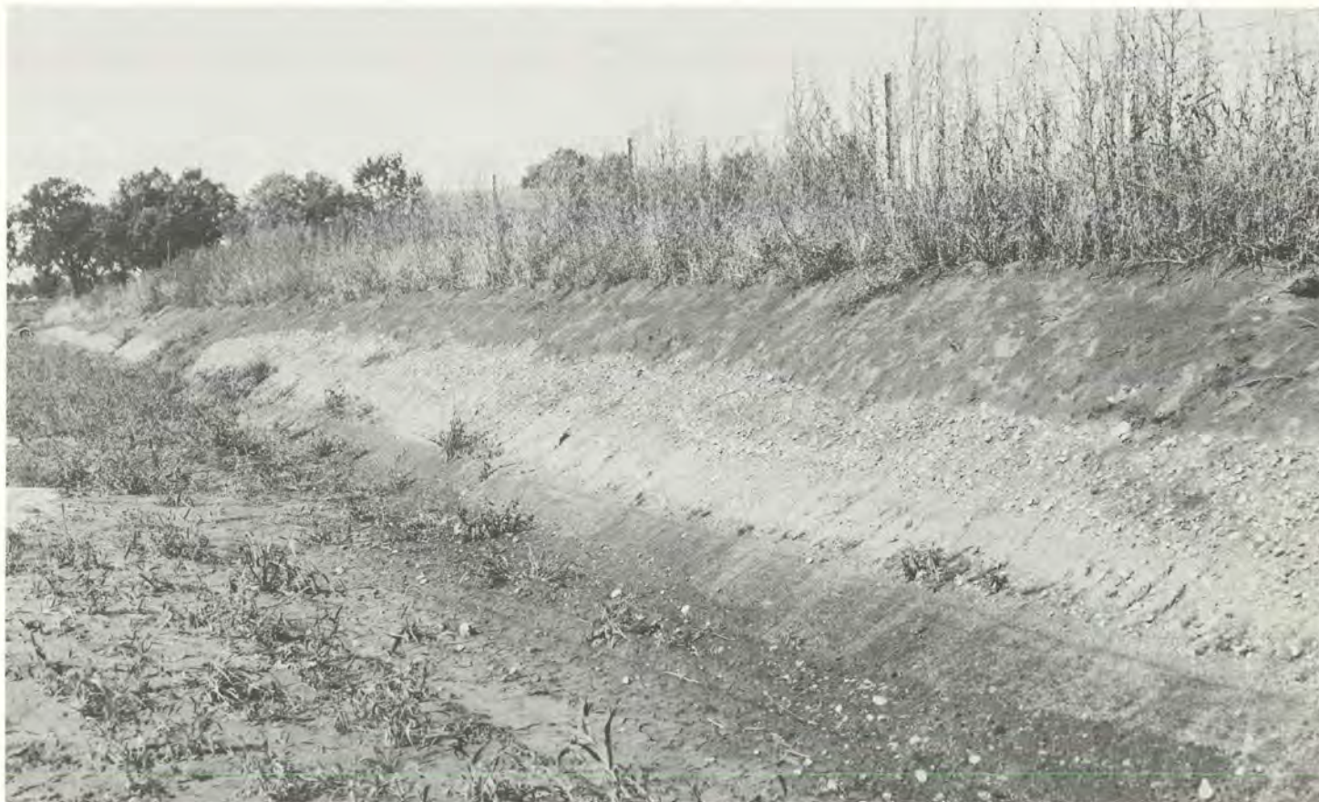
Figure 8.—Saude soils on high alluvial terraces. These soils are underlain by sand and gravel. Permeability is moderate to very rapid. The limitation for septic tank absorption fields is only slight, but contamination of ground water is a hazard.
