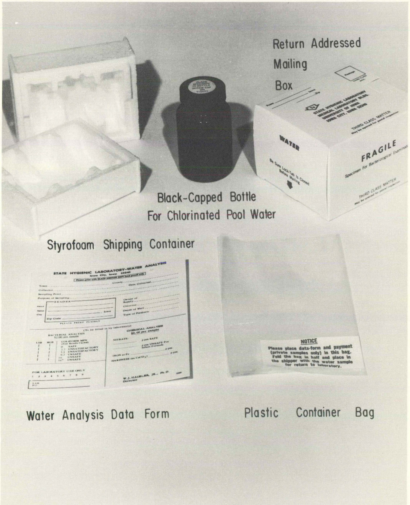
Figure 12-6 Swimming pool water collection kit
