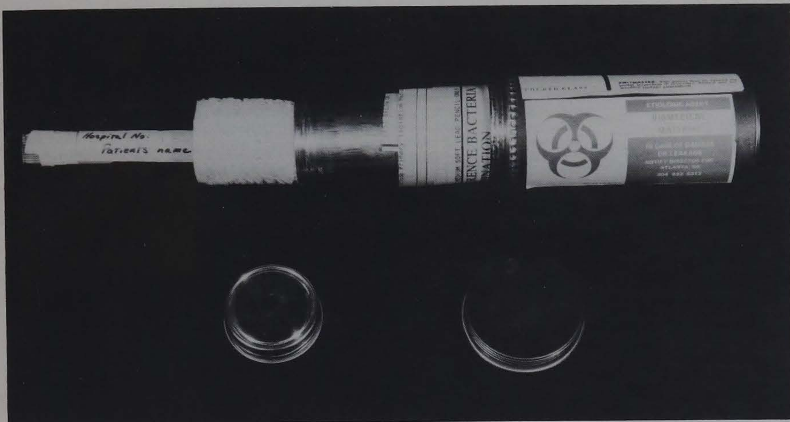
Figure 2-12 Shipping container for reference bacteria specimens
