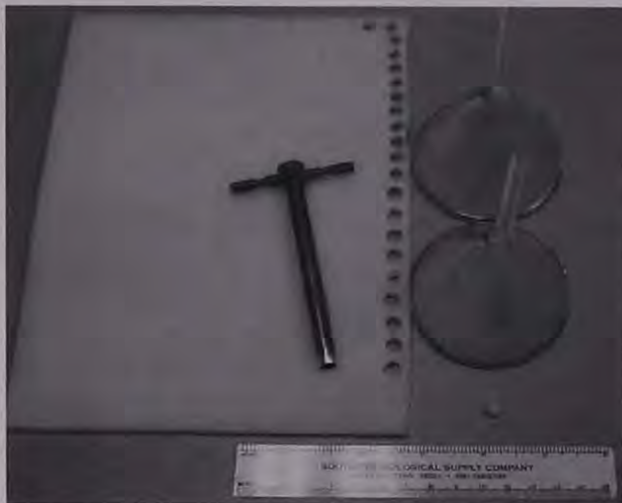
Figure 1. Foam disks cut from foam sheet using a cork borer. Each foam disk is inserted into the stem of glass funnel.
