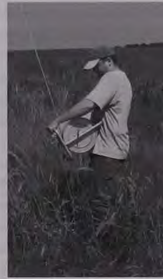
Figure 4. Hand-crank reel used to release and retrieve tetherline to aerial platform.
