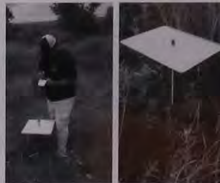
Figure 7. Field markers can serve as easily identifiable reference points in the aerial photographs as well as ground control points when GPS coordinates are obtained. GPS coordinates are necessary for geo-rectification and detailed analysis. The field marker on the left incorporates a tripod support, which allows for adjustment of the marker relative to vegetation canopy (e.g., grasses and forbs).
