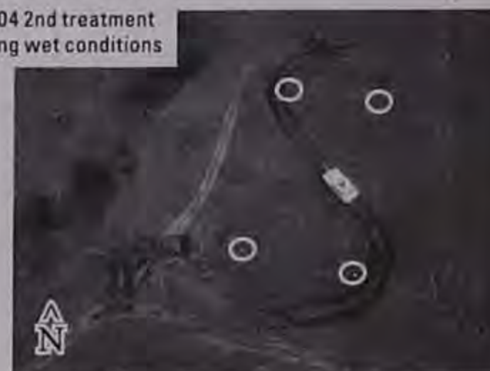
Figure 8. Low-level aerial digital photograph of a tracked-vehicle disturbance treatment in progress. Field markers of known position/distance apart (circled in white) provide ground-control points for photo interpretation and analysis. Markers were 20 cm x 20 cm and photo was taken from an altitude of approximately 90 m (300 ft.).
