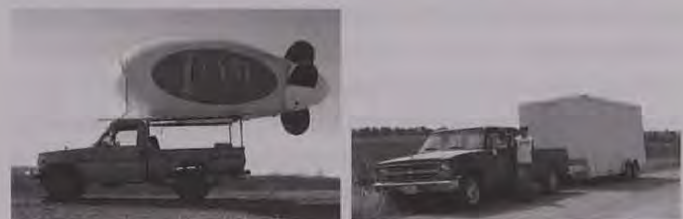
Figure 5. Transportation options for aerial lift platforms. Left: customized rack and netting allowing quick transport from site to site but no off-site storage. Right: box trailer that provides off-site storage as well as transportation to the field of inflated blimp or balloon.
