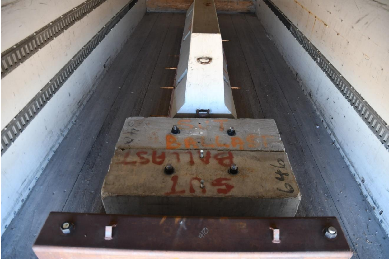
Figure 73. Test Vehicle Ballast, Test No. ABCBRM-1 95
