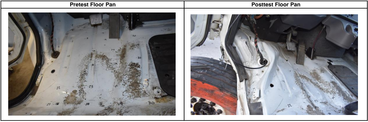
Figure H-2. Floor Pan Deformation Data – Set 2, Test No. ABCBRM-1
