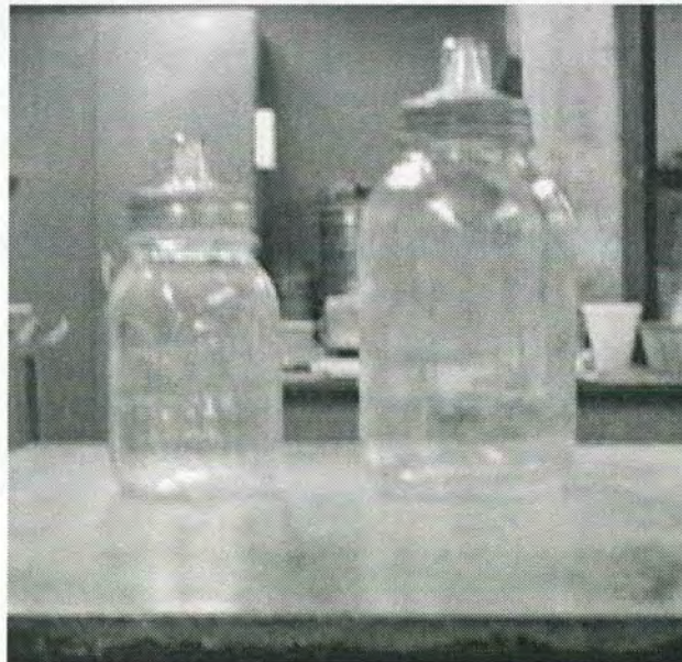
Pycnometers for Coarse and Fine Aggregates
