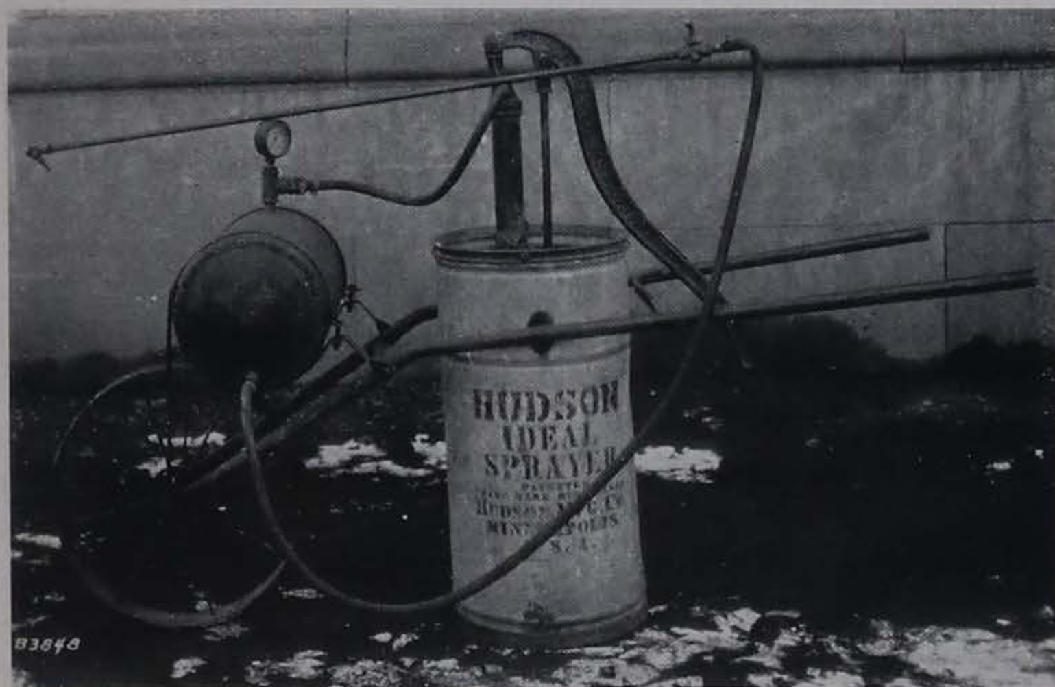
Fig. 11. A wheelbarrow pressure sprayer suitable for weed spraying.
