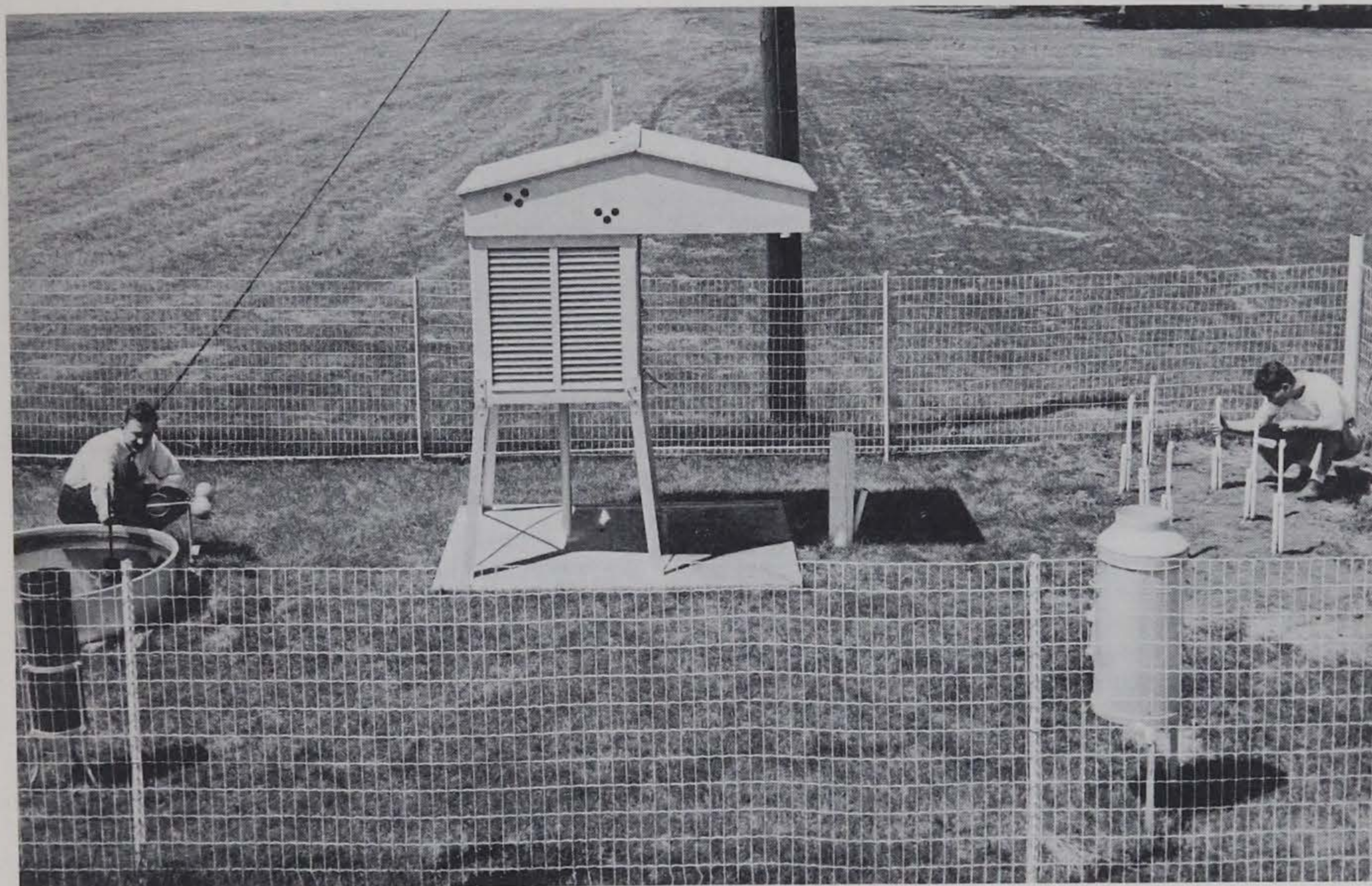
Fig. 1. This weather station at the Iowa State College Agronomy Farm at Ames is more complete than the cooperative observer stations located throughout the state, but it illustrates the type of ventilated shelter in which the thermometers are always exposed and the standard Weather Bureau rain gage in the far left foreground. In addition, this station has a pan for measuring water evaporated and a wind gage immediately above it. In the right foreground is a recording rain gage and behind it are soil thermometers measuring soil temperature at depths from 1 inch to 72 inches below the surface. A psychrometer for measuring humidity is also located inside the shelter.
