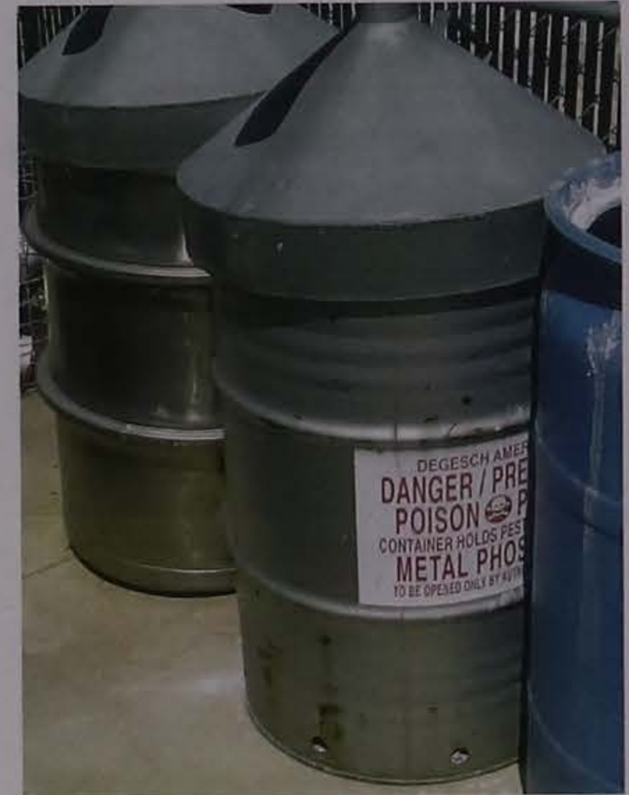
Figure 26. Dry deactivation drum for aluminum and magnesium phosphide deactivation.
