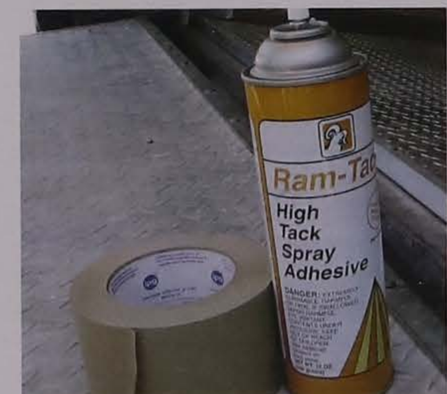
Figure 36. Spray adhesive and tape used in a tape-and-seal fumigation.
