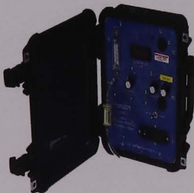
Figure 30. Fumiscope®, a thermal conductivity analyzer, has been used for many years to detect both methyl bromide and sulfuryl fluoride at high concentrations.
