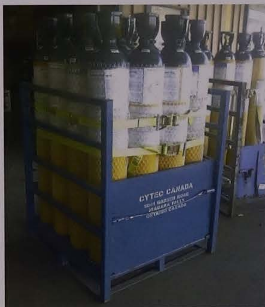
Figure 3. Cylinderized phosphine gas formulation of 2% phosphine plus 98% carbon dioxide.
