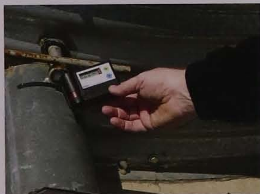
Figure 31. Detecting gas levels outside a grain bin with a low concentration detector.
