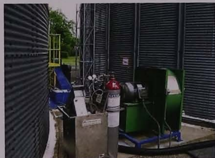
Figure 4. The Hom Diluphos System (HDS) allows the blending of pure cylinderized phosphine gas into air.
