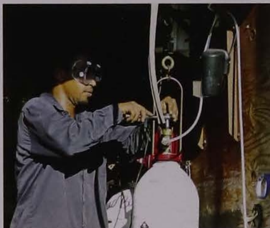
Figure 39. Releasing cylinderized gas through the introduction hose.
