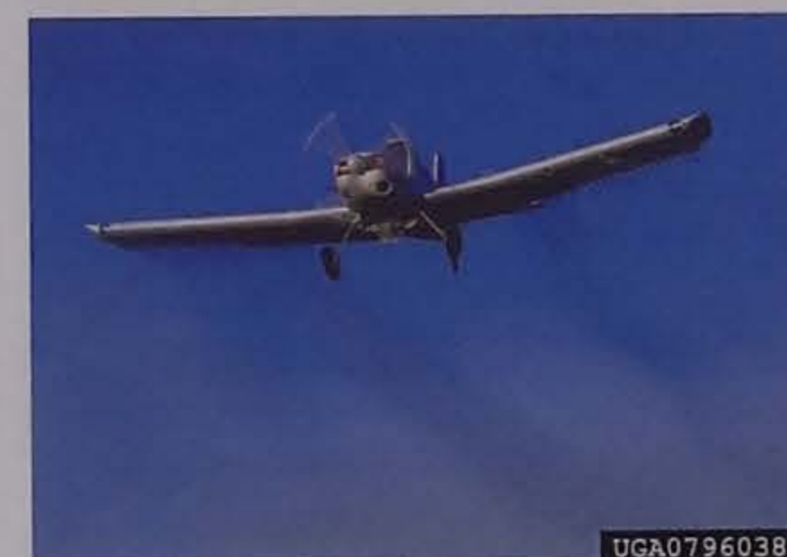
Figure 3.20. Fixed wing aircraft sprayer. Photo credit: Larry Barber, USDA Forest Service, Bugwood.org
