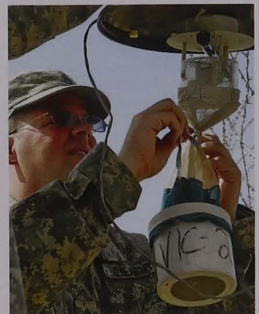
Figure 3.4. Light trap for sampling adult mosquitoes. Photo credit: U.S. Army Photo, Sgt. Joshua Risner, 211 MPAD, MND-B
