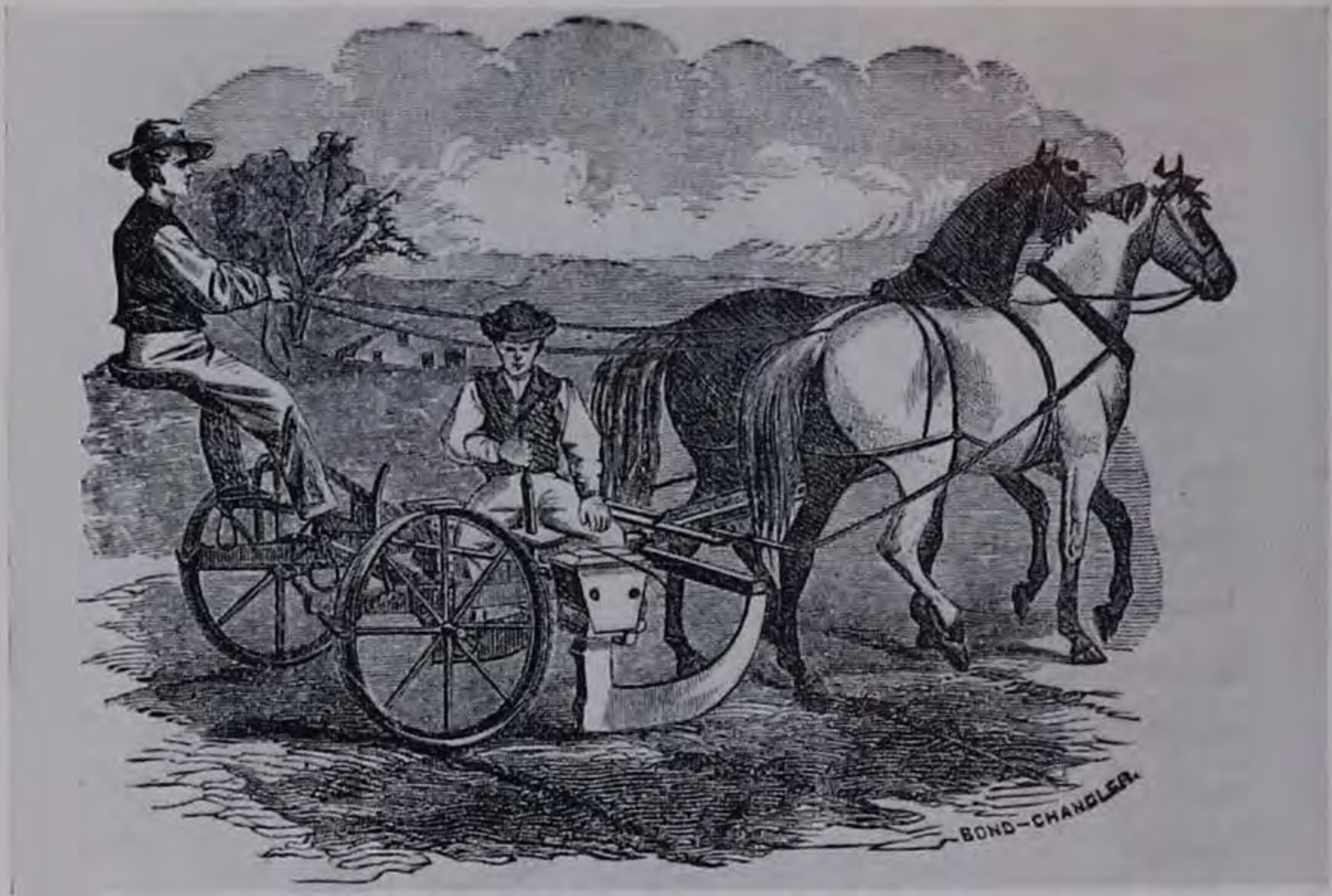
In 1867, 416 of these corn planters were sold in Iowa for seventy dollars each. Two operators were needed, one to drive the team and manage the raising and lowering of the furrow openers, and one to operate the dropping mechanism.—CHAPTER 21, THE ROLE OF MACHINERY IN IOWA FARMING.
