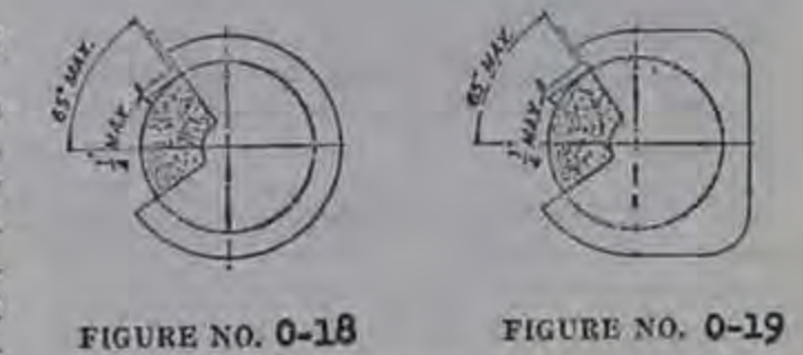
FIGURE NO. O-18 FIGURE NO. O-19 CORRECT Showing adjustable tongue giving required angular protection for all sizes of wheel used.
