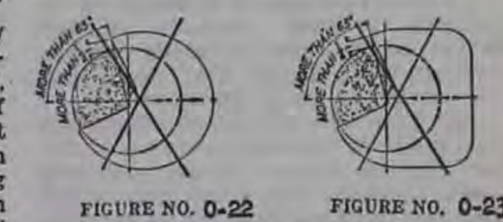
FIGURE NO. O-22 FIGURE NO. O-23 INCORRECT Showing movable guard with size of opening correct for full size wheel but too large for smaller wheels.
