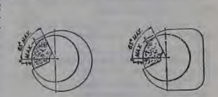
FIGURE NO. O-20 FIGURE NO. O-21 CORRECT Showing movable guard with opening small enough to give required protection for smallest size wheel used.
