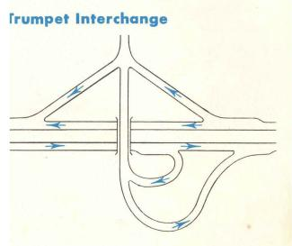
This is a means of providing access to a uperhighway when another roadway connects, orming a "T" intersection. It is a variation of lirectional or diamond type interchange to pernit turning movements on and off the highway.
