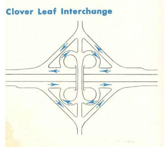
An interchange designed to allow turning movements off or onto the Interstate from four directions using loop type connections. It eliminates left turn and cross traffic conflicts for all movements. Some partial cloverleaf designs have loops in two or three quadrants.
