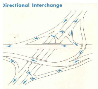
This type of interchange is used where a high olume of traffic desires to transfer between only wo legs of the interchange. The high volume f left turn movements from the west to the orth are made by a directional ramp. Other novements are accomplished by the conventional iamond type ramps. This type is now in use at he interchange between Interstate 80 and U. S. 5 and Iowa 64 northeast of Des Moines.
