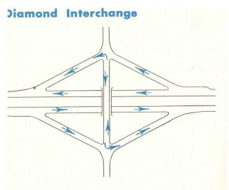
An interchange, characterized by four ramps, which allows vehicles to enter or leave the main highway while flowing with the traffic. Left turns are made at grade on the crossroad.
