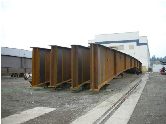
Figure 17 Example of bridge girders
