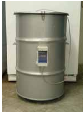
Figure C4. Semi-adiabatic calorimeter–IQ drum ( www.quadreliservice.com )
