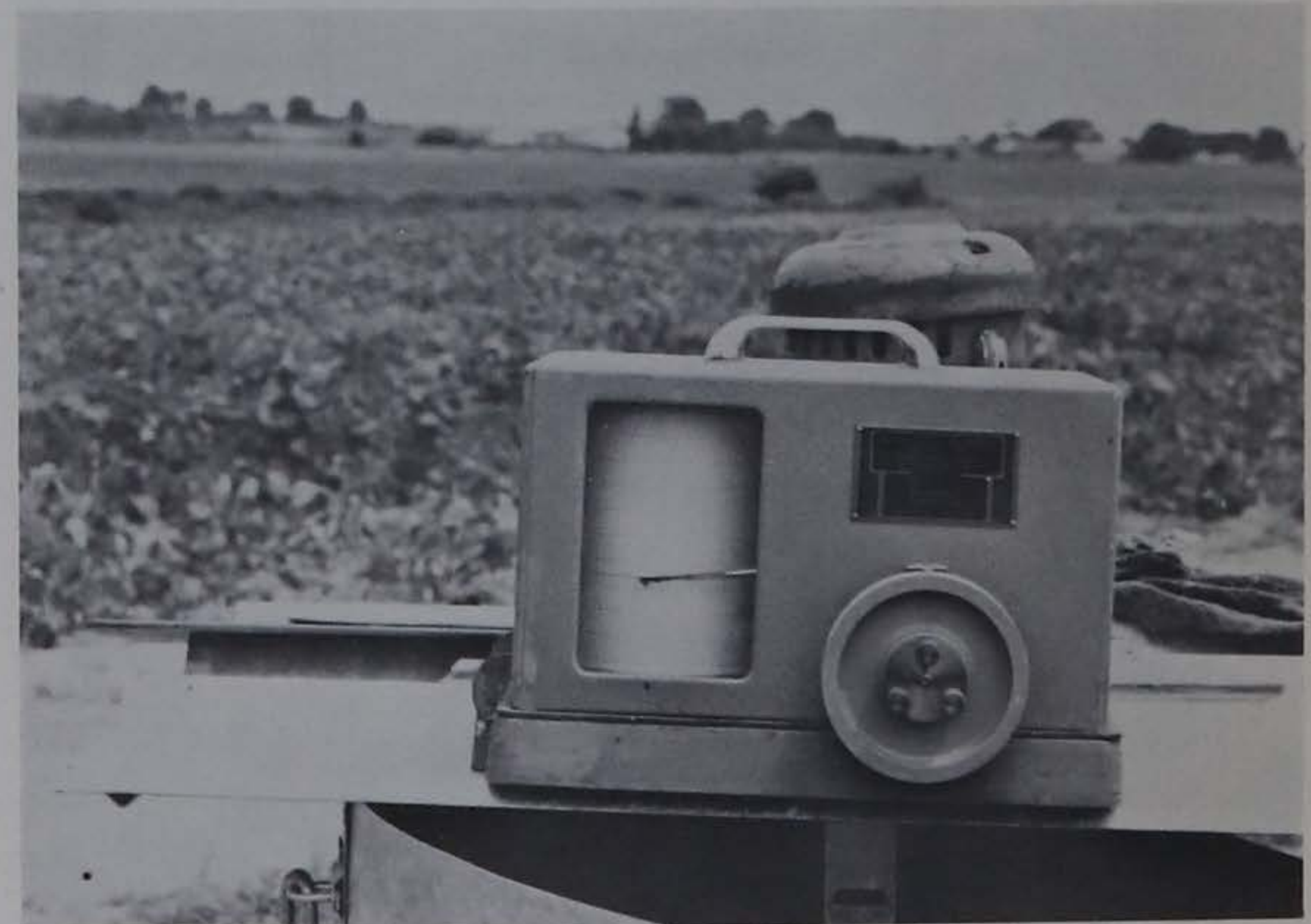
Water level recorder
