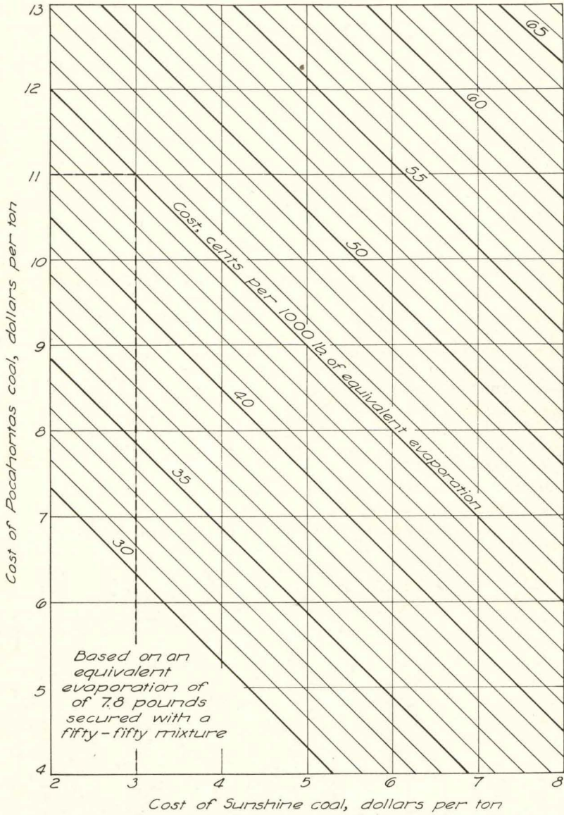
Fig. 13.—Cost of heating with a fifty-fifty Sunshine-Pocahontas coal mixture. Only the cost of coal is considered.
