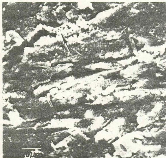
Figure 6. Fracture pattern through a deposit of pyrite crystallites in chemically comminuted coal of region 1 in Figure 5. Pyrite crystals are indicated by the arrow.
