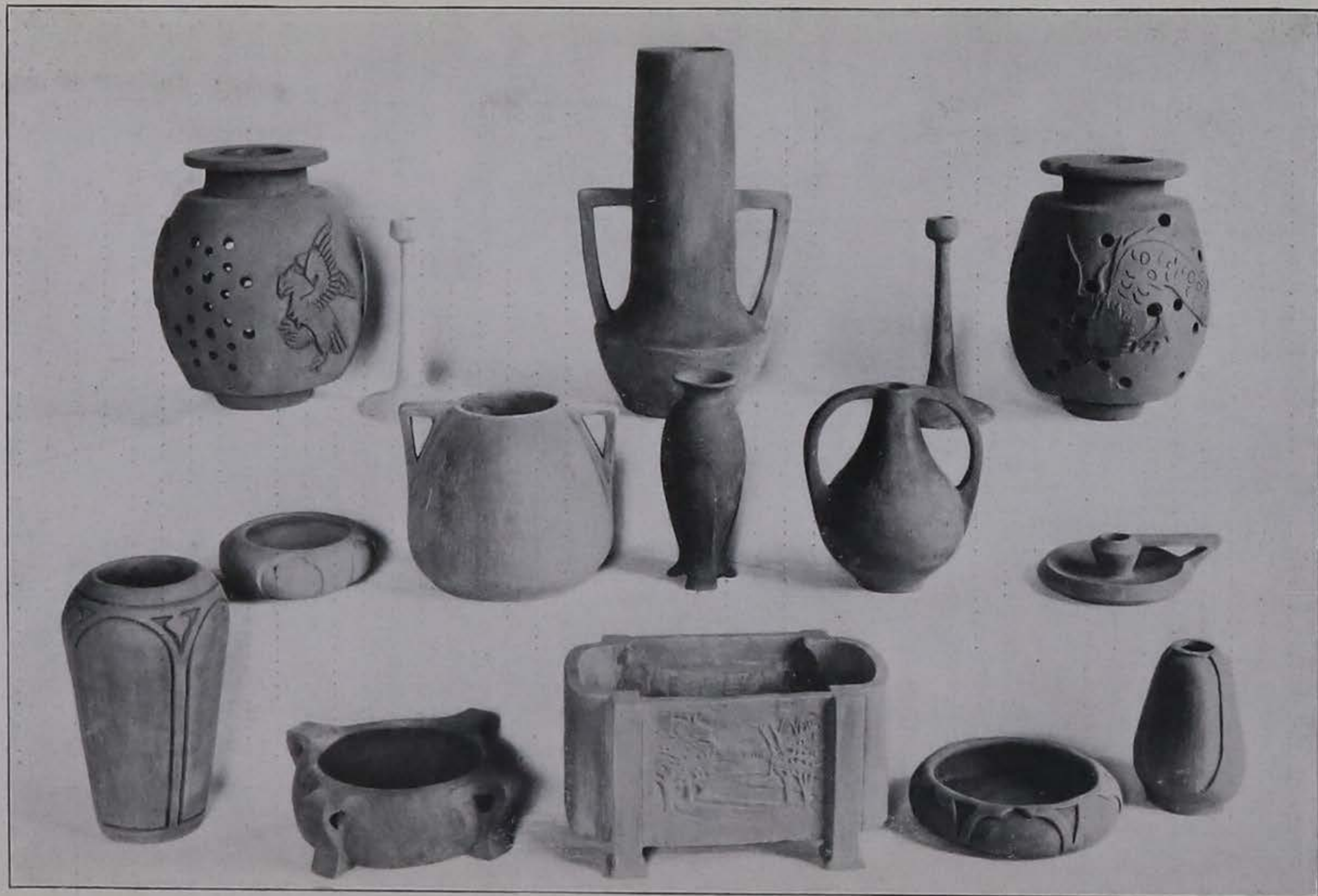
FRONTISPIECE. SHOWING PIECES MADE FROM IMPROVED IOWA SHALE. The body for these pieces was 80 per cent Mason City Shale and 20 per cent Mason City Yellow Clay.
