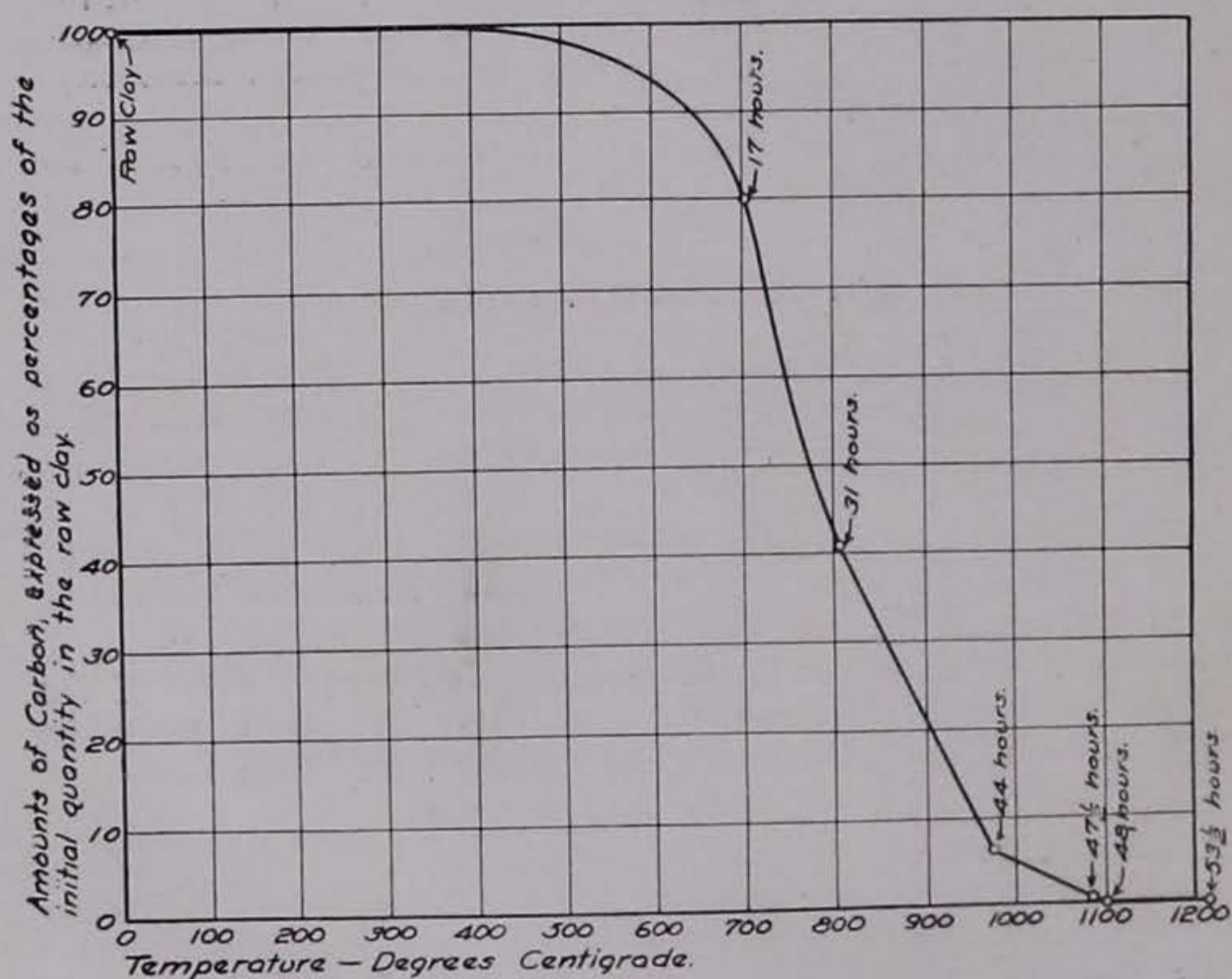
Fig. 1. Curve showing the oxidation of carbon in the burning of a clay.
