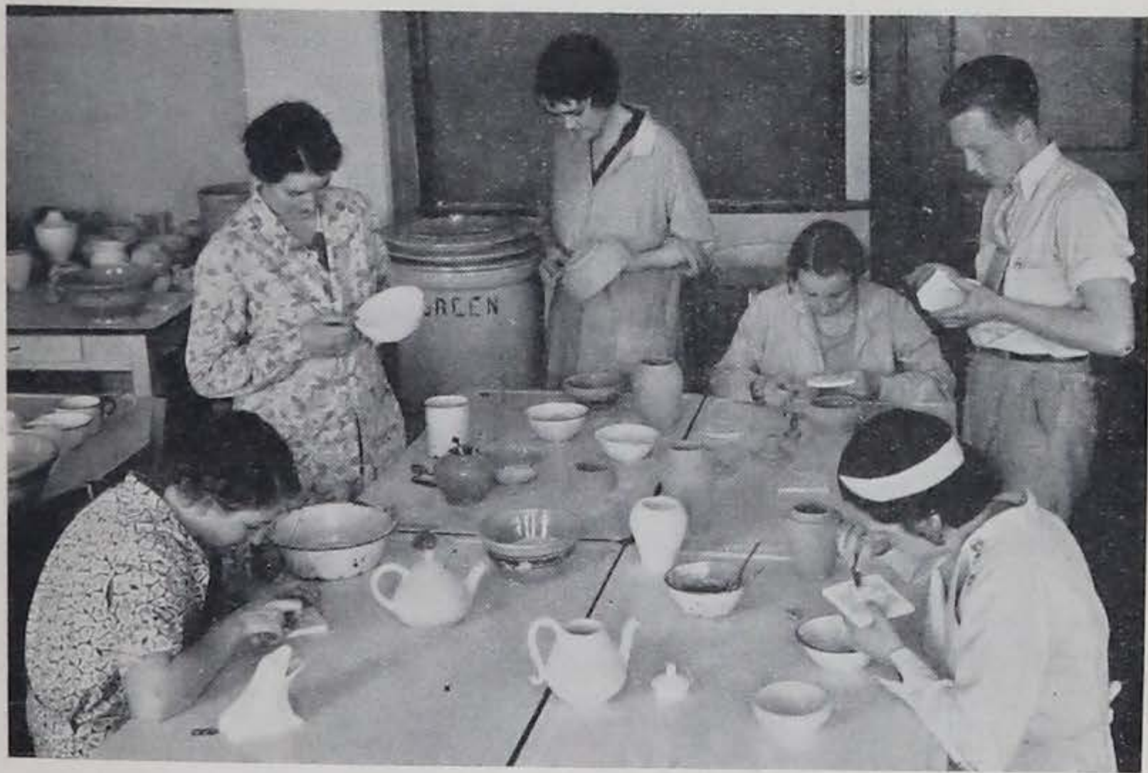
Fig. 16.—The wares pictured above have been dipped in the glaze jars shown in the background. Some of the students are evening the glaze layers, while others are applying glazes of other colors by means of brushes, knives, and medicine droppers.
