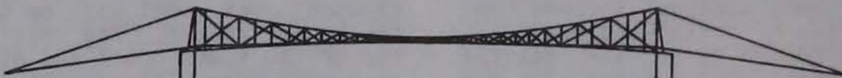
Figure 2 Modified Patterson Loop Aerial Crossing
