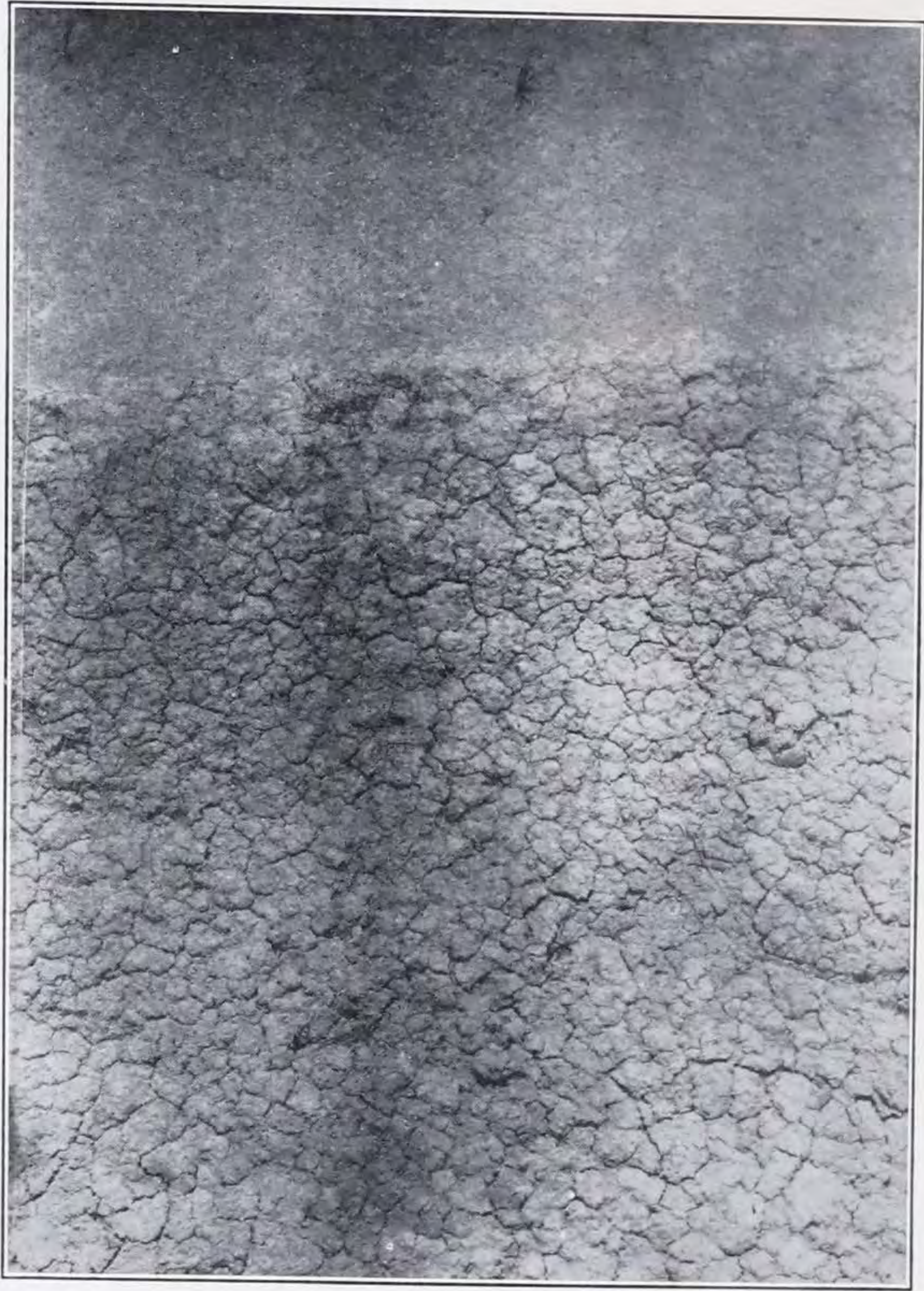
FIG. 35.—Showing dried surface of gumbotil with smooth loess surface above it. Both materials have had the same amount of exposure.
