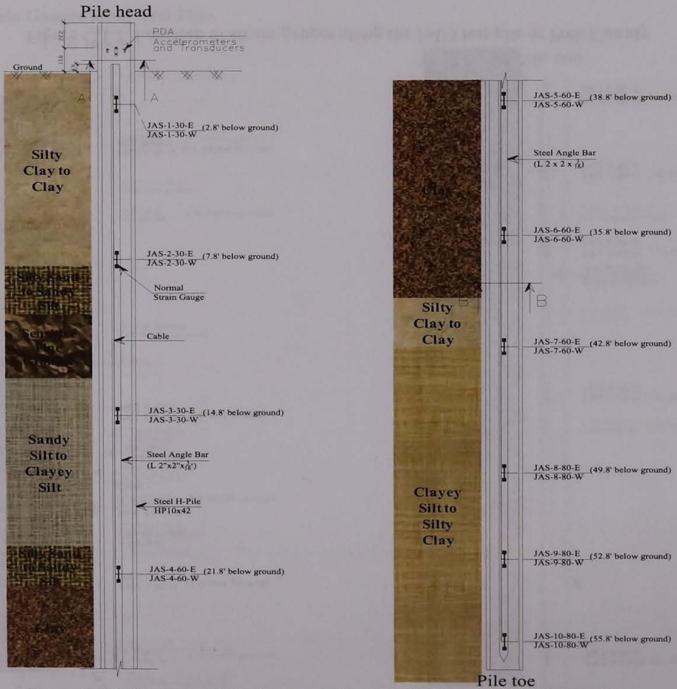
Figure C.1.3. Location of strain gauges along the ISU4 test pile at Jasper County
