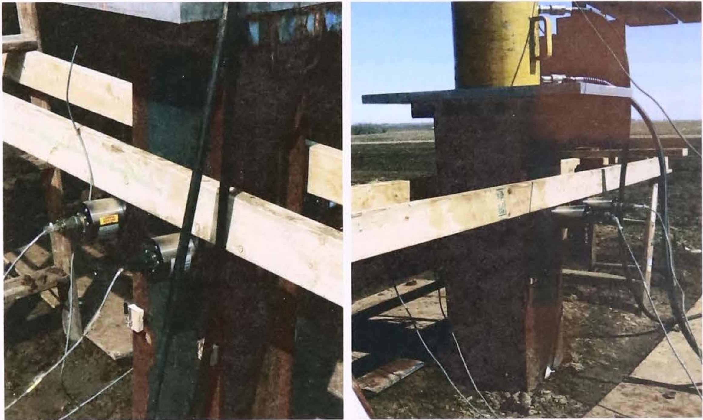
Figure 4.20. Pile top vertical displacement transducers instrumentation
