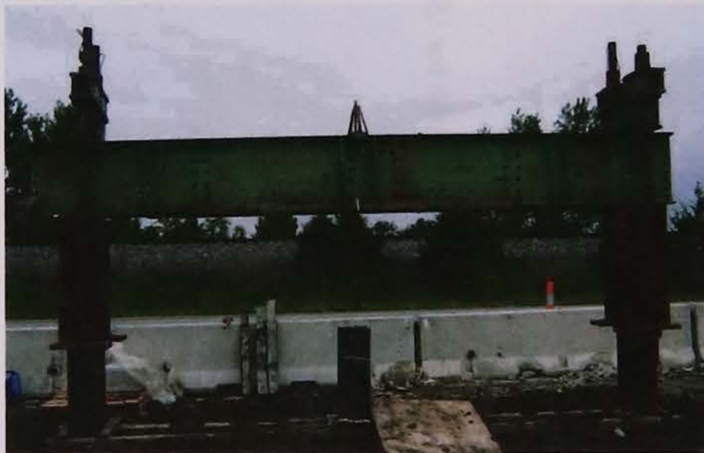
(c) Assembled a main reaction beam, clamping beams and height adjusters; Fastened with steel rods
