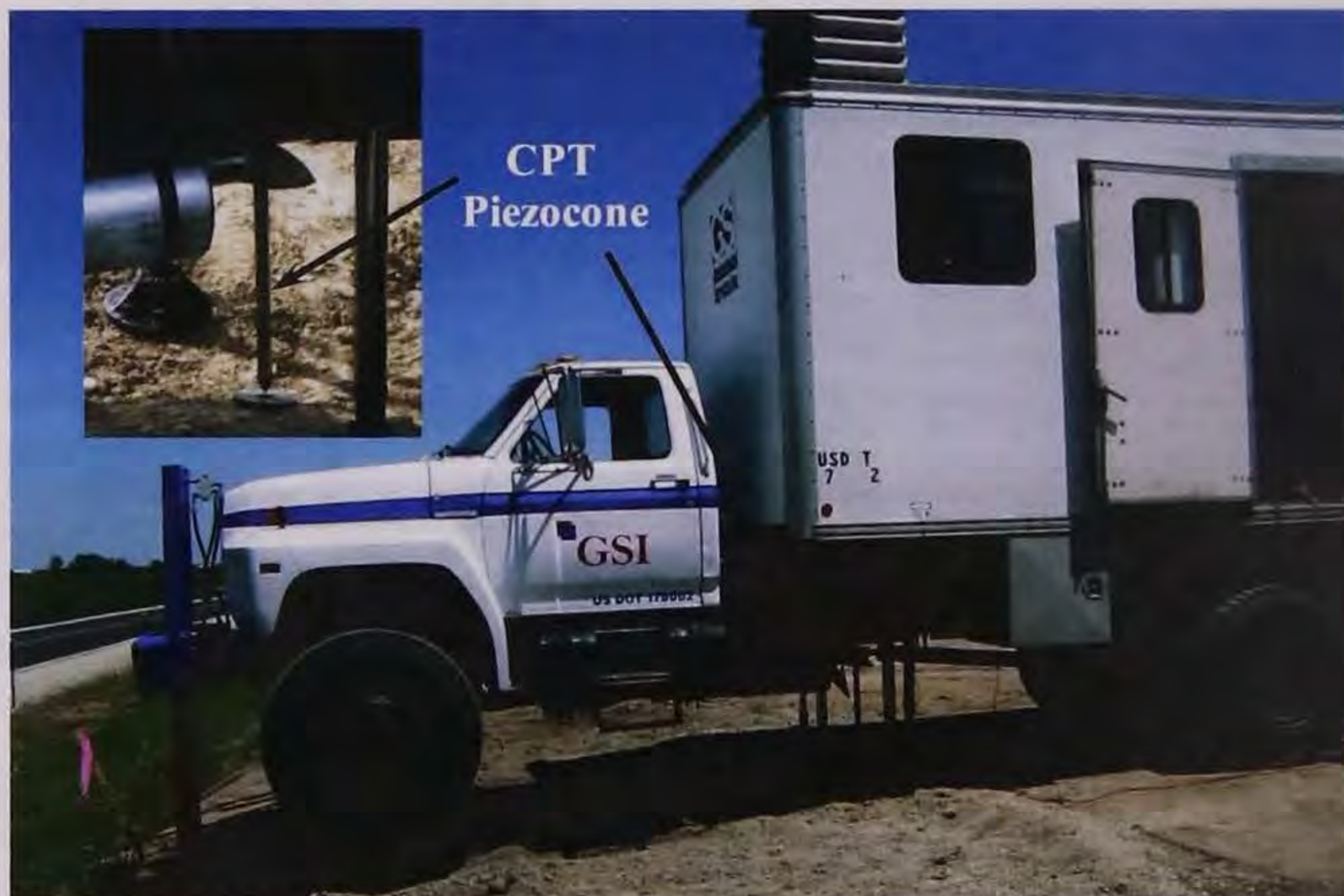
Figure 3.3. Typical Cone Penetration Test (CPT)
