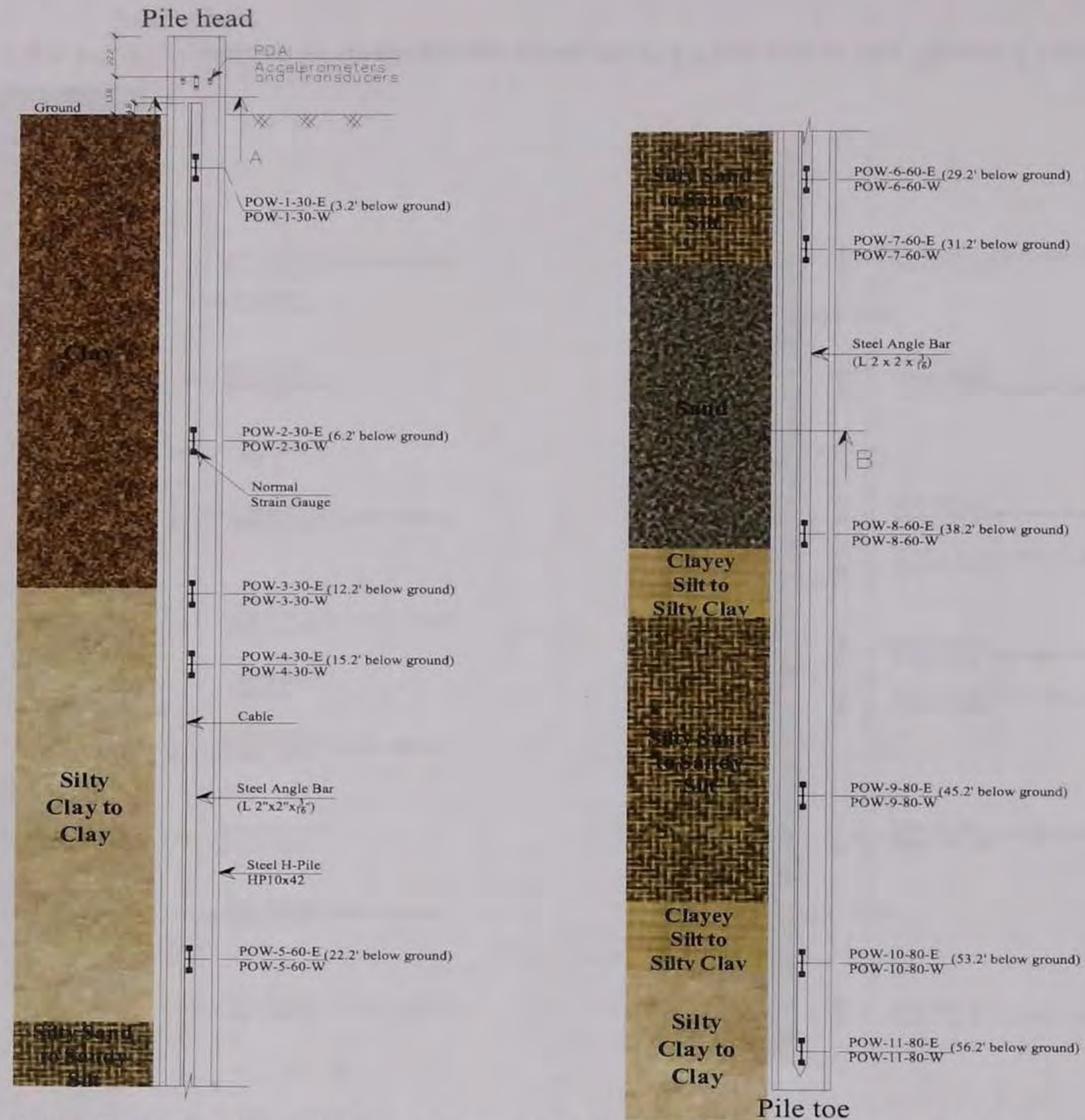
Figure C.1.6. Location of strain gauges along the ISU8 test pile at Poweshiek County
