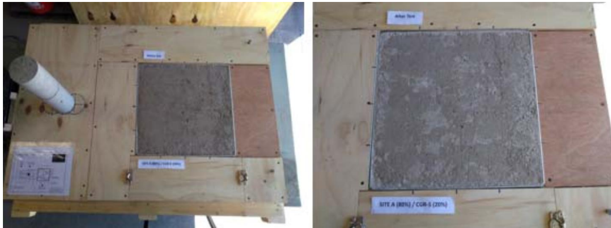
Figure 39. Views of WETA and compacted soil form during wind erosion test
