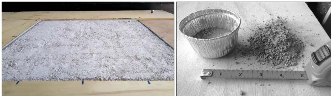
Figure 40. Soil loss due to wind erosion from compacted soil form (left) and loose eroded fines (right)
