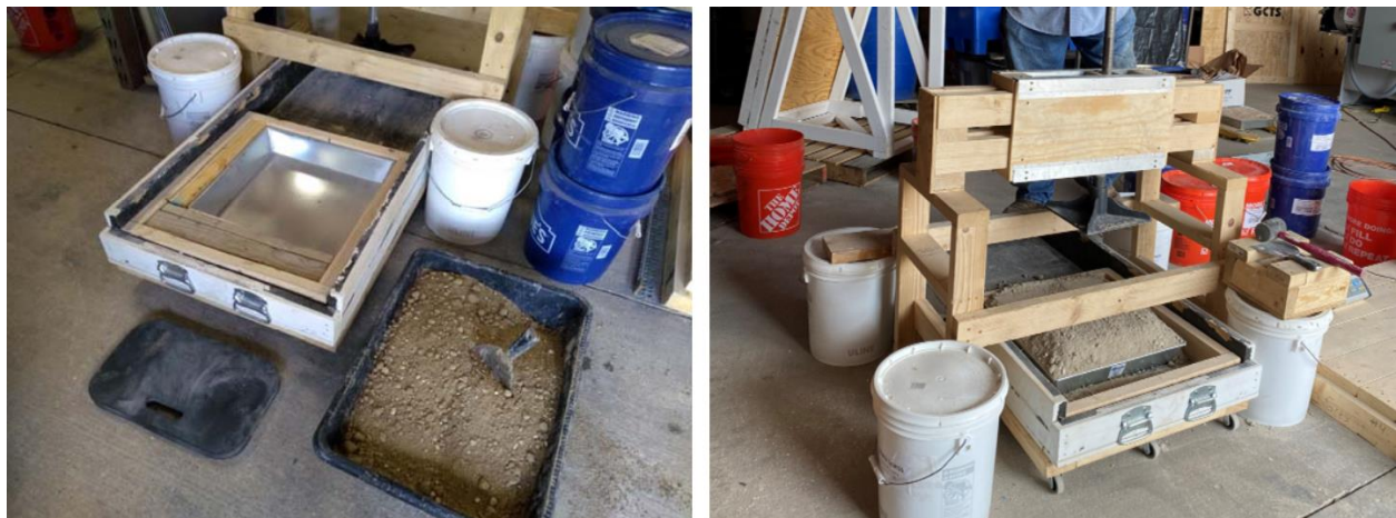
Figure 36. Steps during compaction of soil forms using UTA
