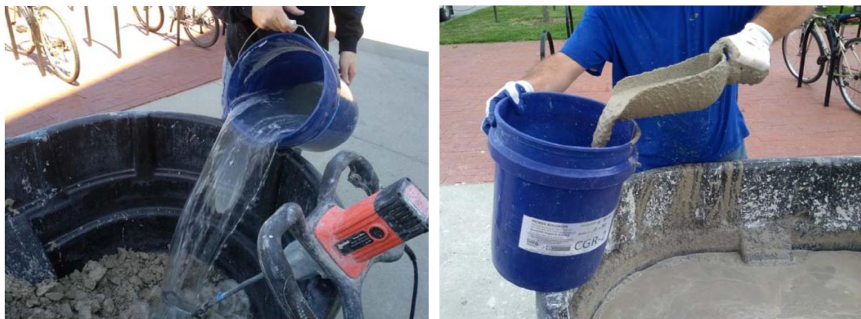
Figure 5. Water being added to CGR solids (left) and consistency of homogeneous CGR slurries (right)
