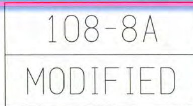
Figure 5: The box in upper right hand corner of modified design or tabulation form should appear similar to above.
