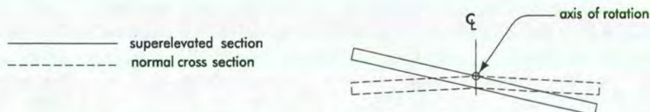
Figure 1: The axis of rotation for undivided highways.
