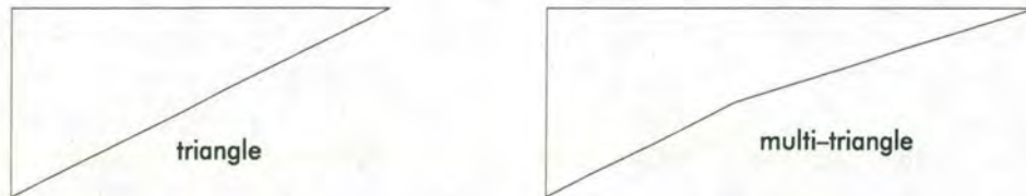
Figure 1: Types of gutter sections.
