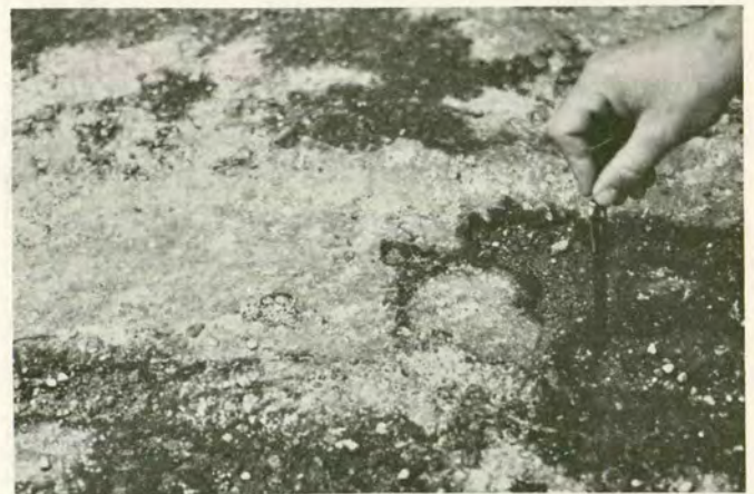
d. Section 5, coherex over previously applied lignosulfonate.
