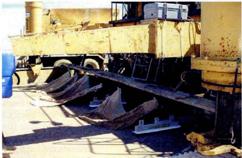
Real Time Profiler Beams Attached in Each Wheel Track
