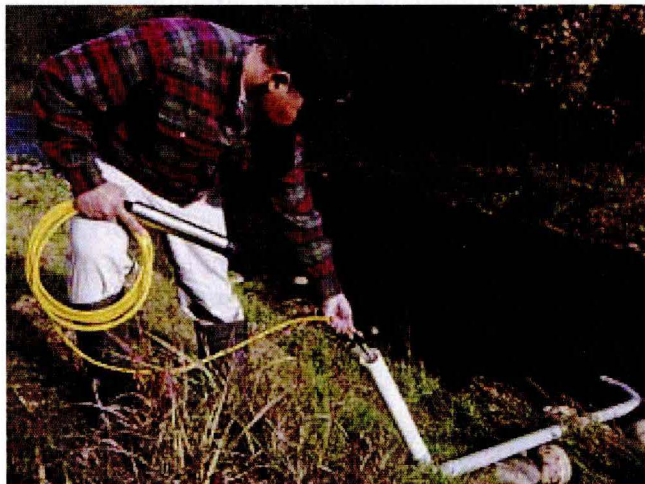
Installation of Water Level Loggers(left) and drawing (below) of Logger Placement
