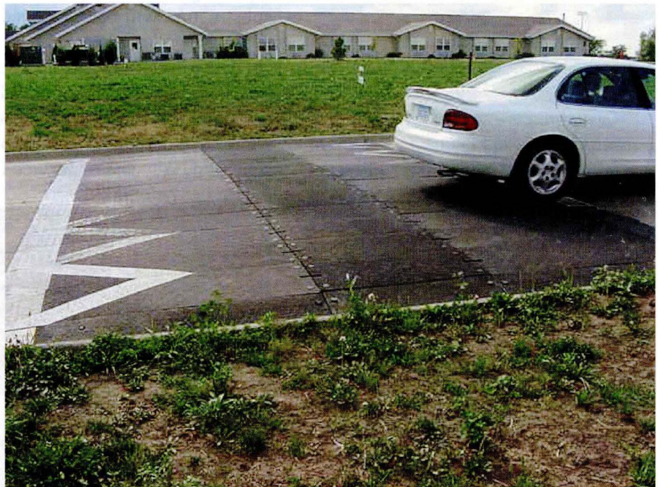
An example of a 30 mph speed table used in CTRE study for residential traffic calming in small Iowa communities.
